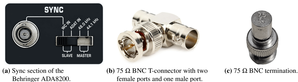
Figure 6: Physical components used for clock synchronization for the Behringer ADA8200 converters and in the cascaded BNC word-clock connections.
