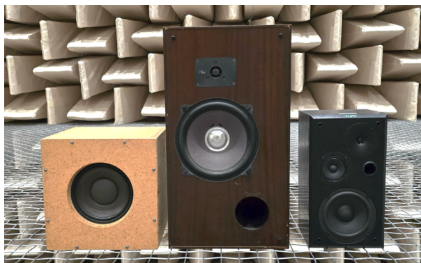
Figure 2: DUTs: DIY Woofer (left), ATR Hifi Speaker (center), Eltax Century 150 (right)
