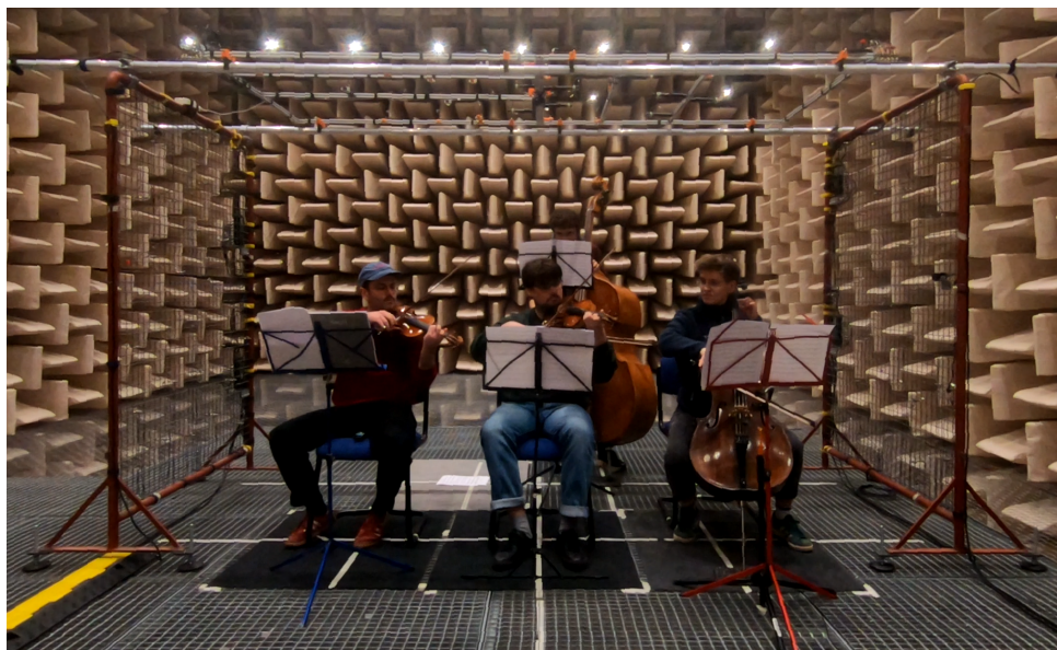
Figure 2: Photograph of the measurement setup with the four instrumentalists inside the anechoic room at the Technische Universität Berlin.
