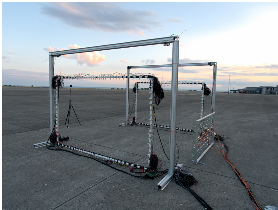
Figure 1: Experimental setup on the apron of Cochstedt-Magdeburg Airport. The two sound sphere array frames as well as the tracking array (right) can be seen. The higher beams are for the cameras of the optical motion tracking system.
