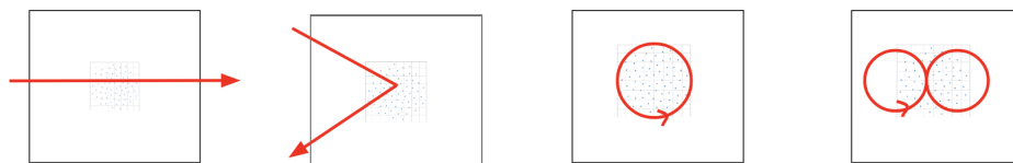
Figure 4: Representations of the measured flight trajectories from left to right: straight, deploy and depart, circling, and figure eight
