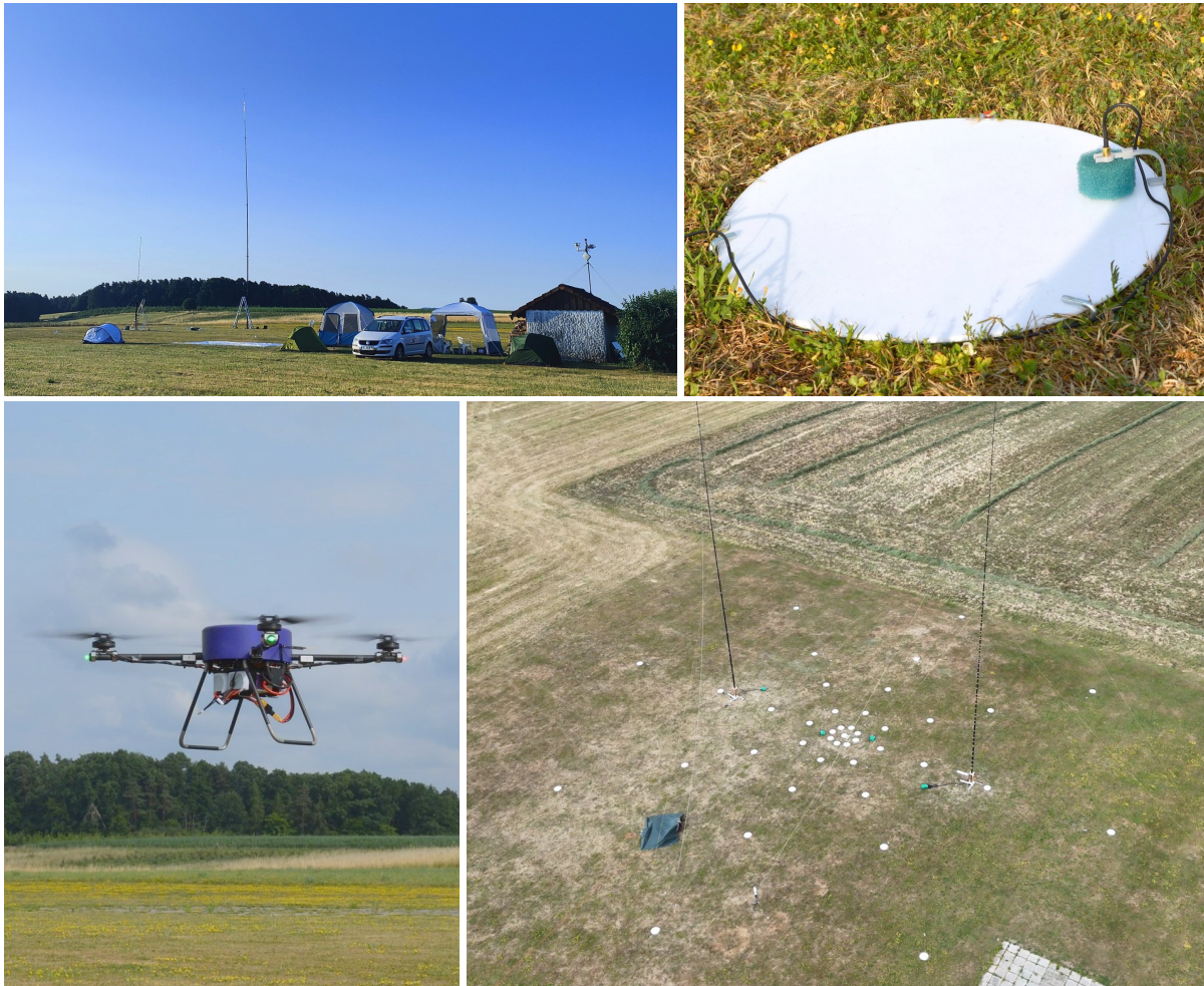
Figure 1: From upper left: in-progress setup of the array, with the transport vehicle for the measurement hardware and accommodation for three people (TUB). Ground plate with one inverted 1/4" microphone. Measured quadcopter (custom-built, FAU). Aerial view of the finished array setup.
