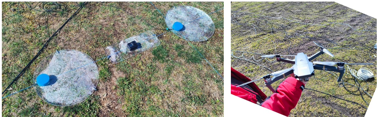
Figure 2: Left: Two microphone ground planes with windscreen and camera for flyover recording. Right: Drone used for the measurement evaluated here.
