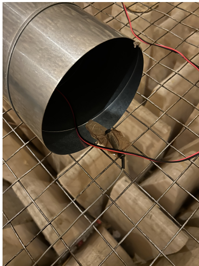
Figure 2: The reference microphone is placed at the exit of the pipe.
