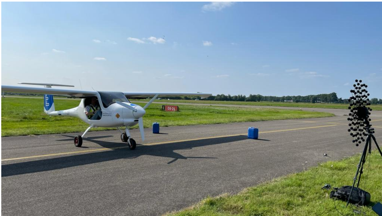
Figure 3: Setup engine run-up with the microphone array aligned with the propeller rotation centre.
