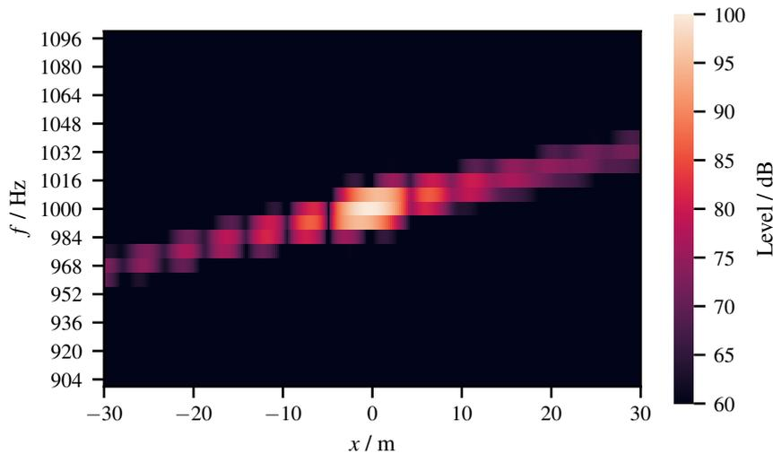
Figure 1: Beamforming results of a monopole at altitude 200 m and  $v_x = 80$  m/s. The source is a tonal source with 1 kHz and 100 dB. The line array consists of 101 equally spaced microphones, For demonstration purposes, the geometric setup replicates the beamforming pattern in [5].
