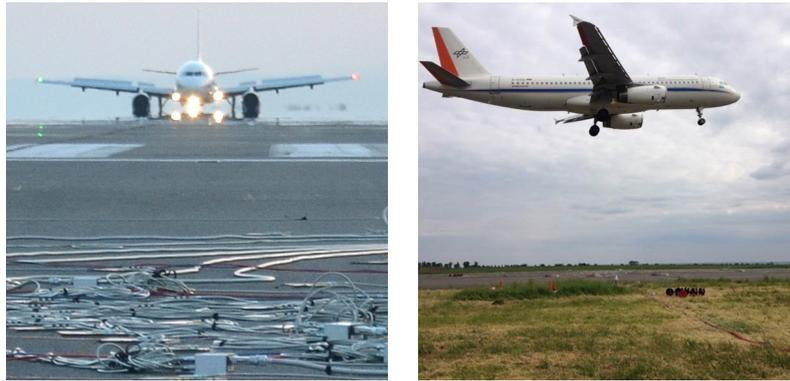
Figure 1: Left: The microphone array with the ATRA in the background. Right: The ATRA flying over the microphone array.
