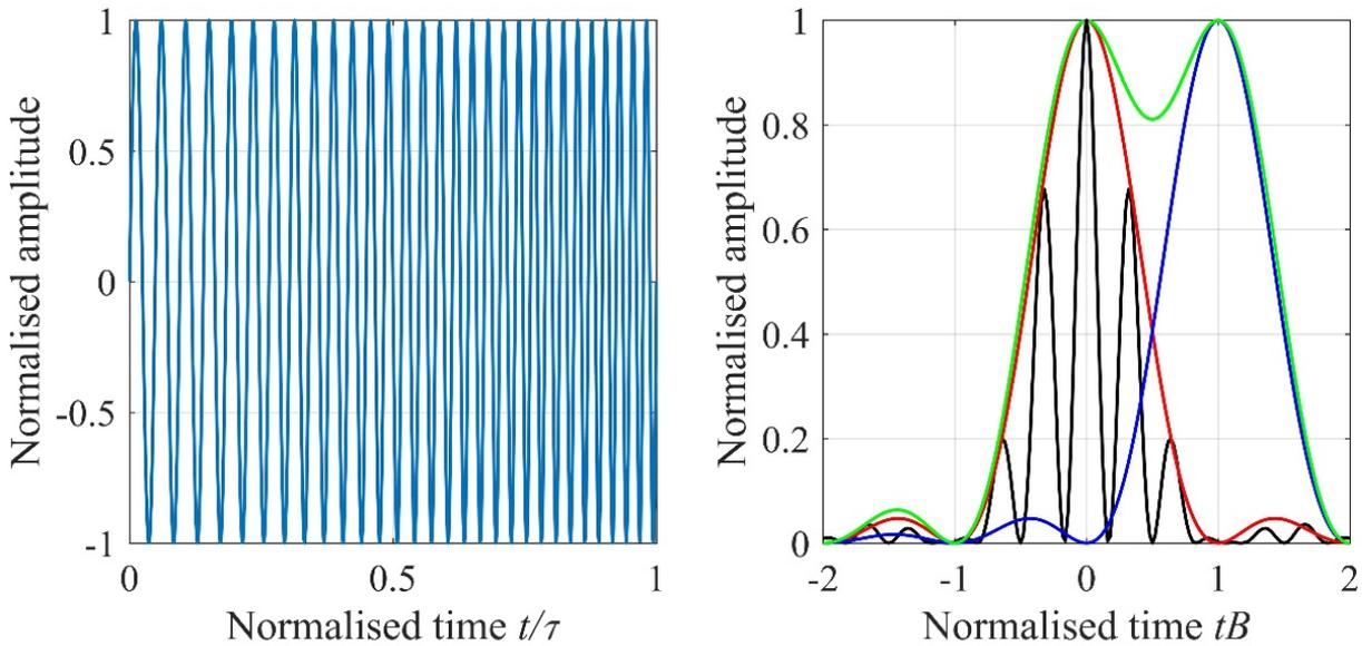
Fig. 1. An example of a linear chirp signal with  $f_0\tau = B\tau = 20$ . The transmitted signal (a), and (b) the square of the correlation of transmitted and received signals (black), the envelope (red), a delayed echo (blue), and the combination of non-delayed and delayed echoes (green).
