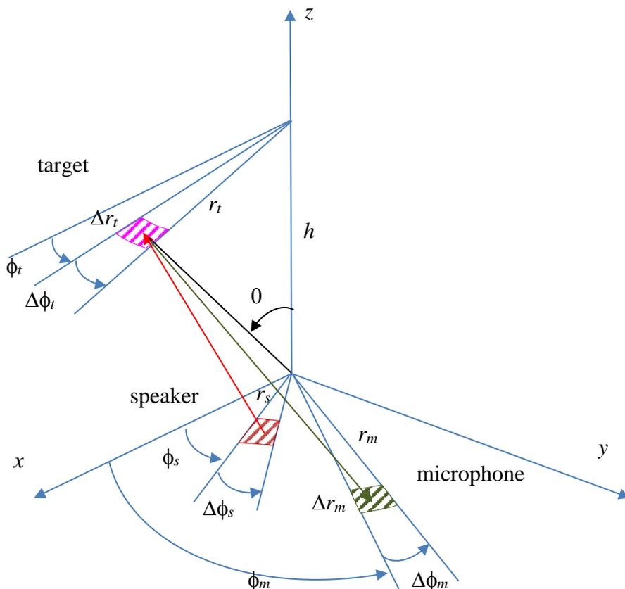
Fig. 2. The general geometry from transmission from a small element on the  $z = 0$  plane, reflection from a small element on the  $z = h$  plane, and reception at a small element on the  $z = 0$  plane.
