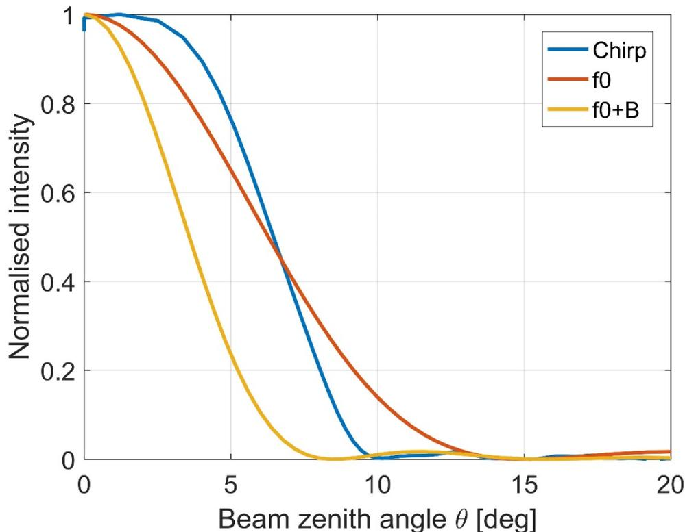
Fig. 5. Plot of intensity as a function of beam zenith angle  $\theta$  for transmission and reception of a chirp pulse (blue), and the corresponding Airy patterns for the base frequency (orange) and the maximum frequency (yellow).
