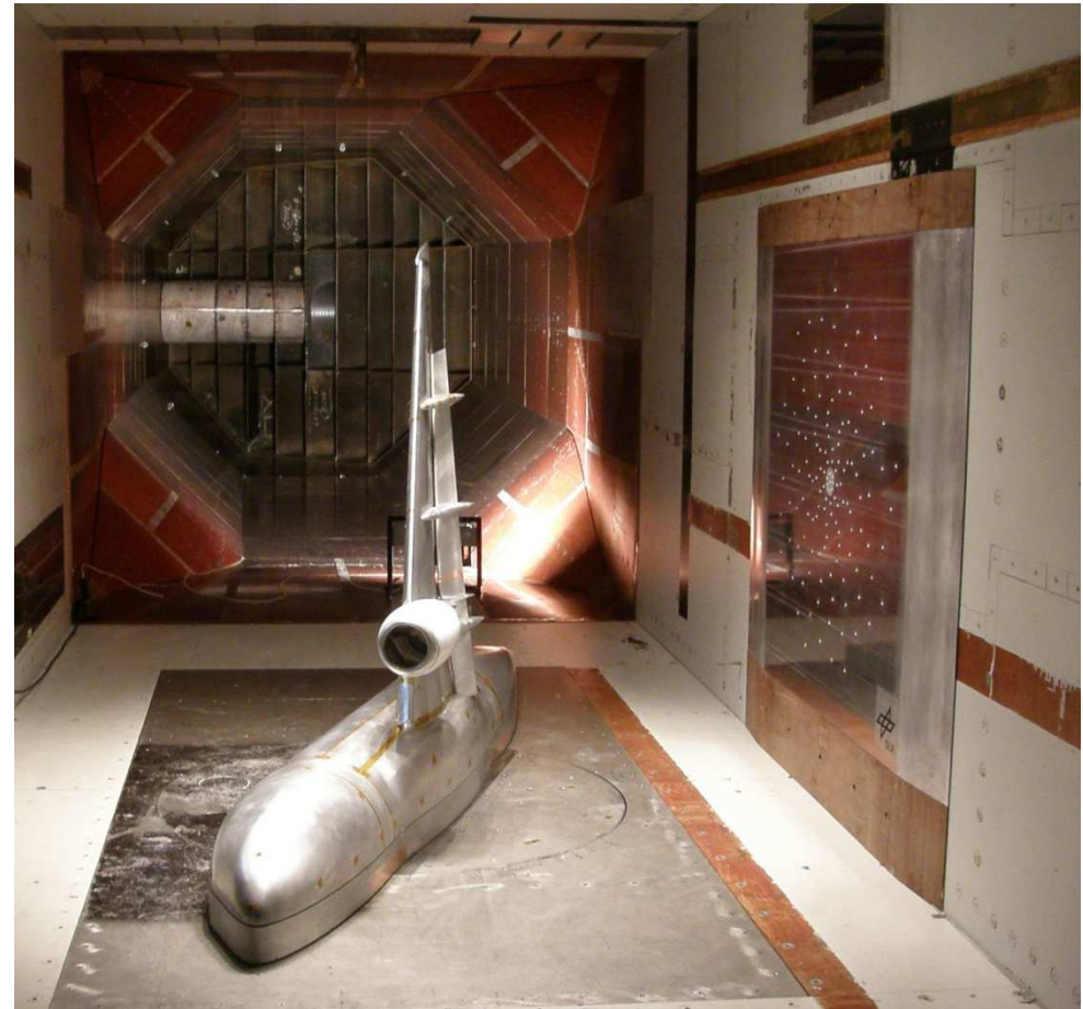
DO-728 half-model at landing configuration
