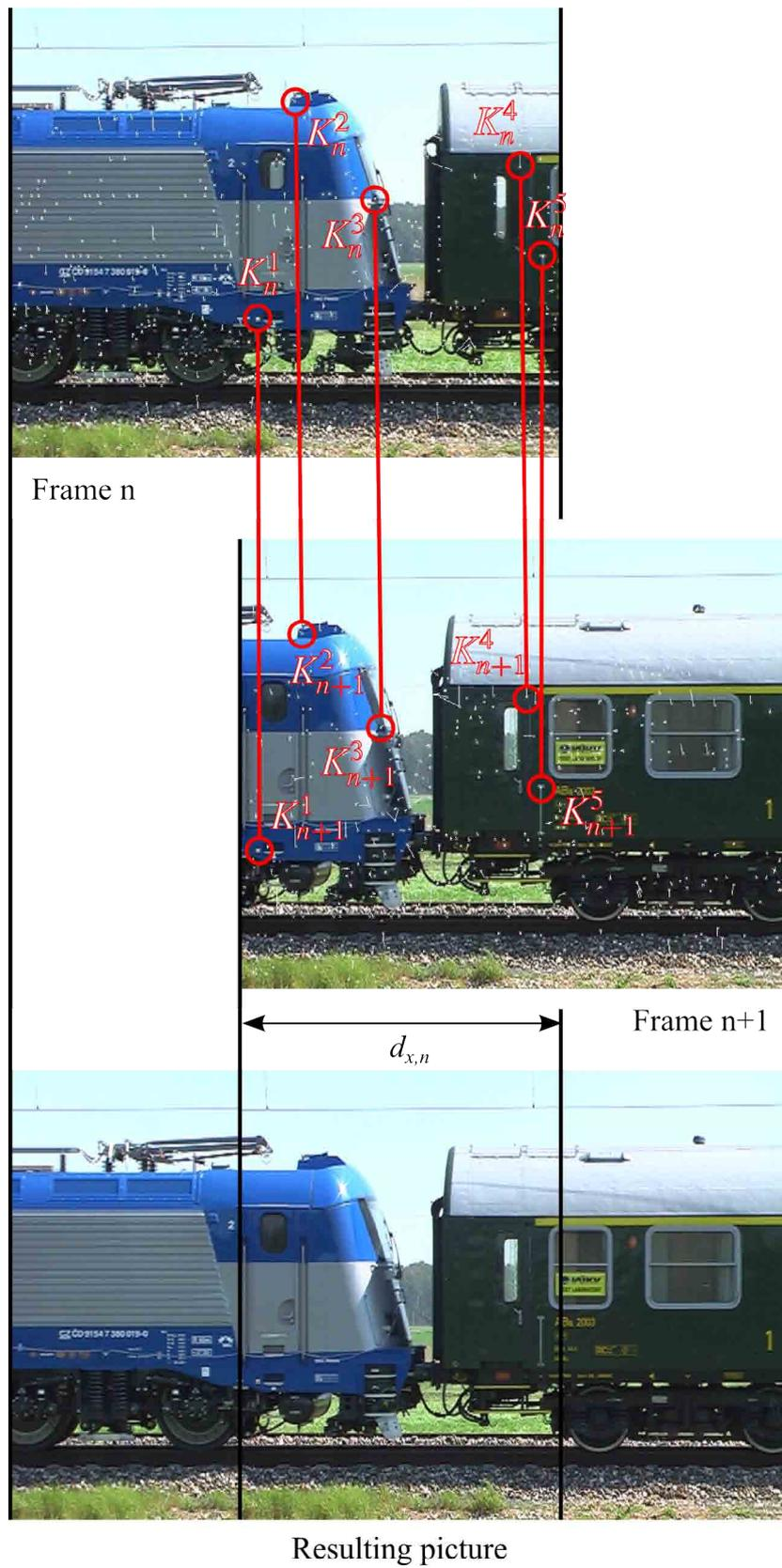
Figure 1: Stitching two adjacent frames  $F_n$  and  $F_{n+1}$  according to their distance  $d_{x,n}$
