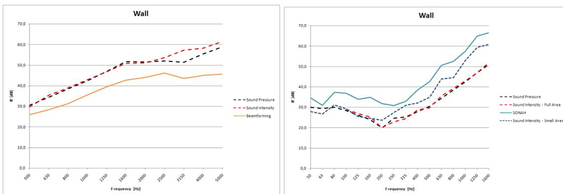
Figure 6: Comparison of sound reduction indexes for the wall. Left: Beamforming. Right: SONAH.
