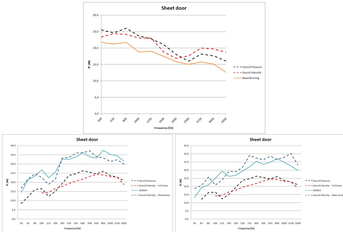
Figure 8: Comparison of sound reduction indexes for the sheet door. Up: Beamforming. Bottom Left: SONAH in the sheet surface. Bottom right: SONAH in the glass surface.
