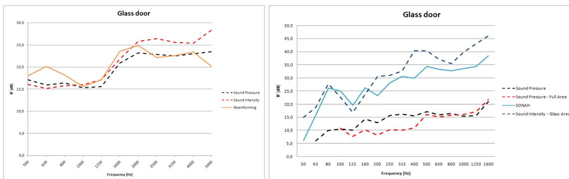
Figure 7: Comparison of sound reduction indexes for the glass door. Left: Beamforming. Right: SONAH.
