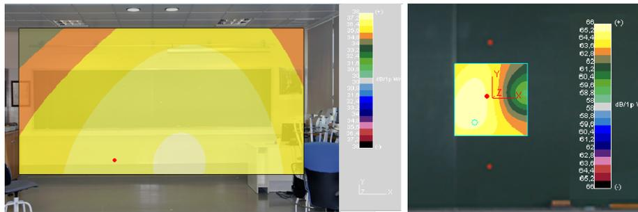
Figure 2: Results for the wall. Left: Beamforming at the third-octave band of 1 kHz. Right: SONAH at the third-octave band of 250 Hz.
