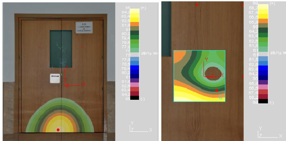
Figure 5: Results for the wooden door. Left: Beamforming at the third-octave band of 500 Hz. Right: SONAH at the third-octave band of 250 Hz.
