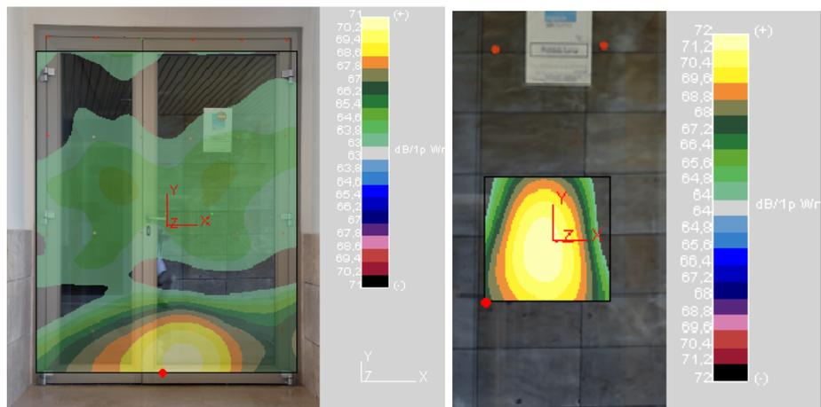
Figure 3: Results for the glass door. Left: Beamforming at the third-octave band of 4 kHz. Right: SONAH at the third-octave band of 160 Hz.
