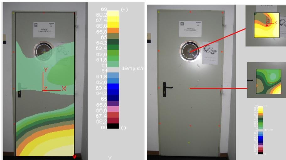
Figure 4: Results for the sheet door. Left: Beamforming at the third-octave band of 2 kHz. Right: SONAH at the third-octave band of 250 Hz.
