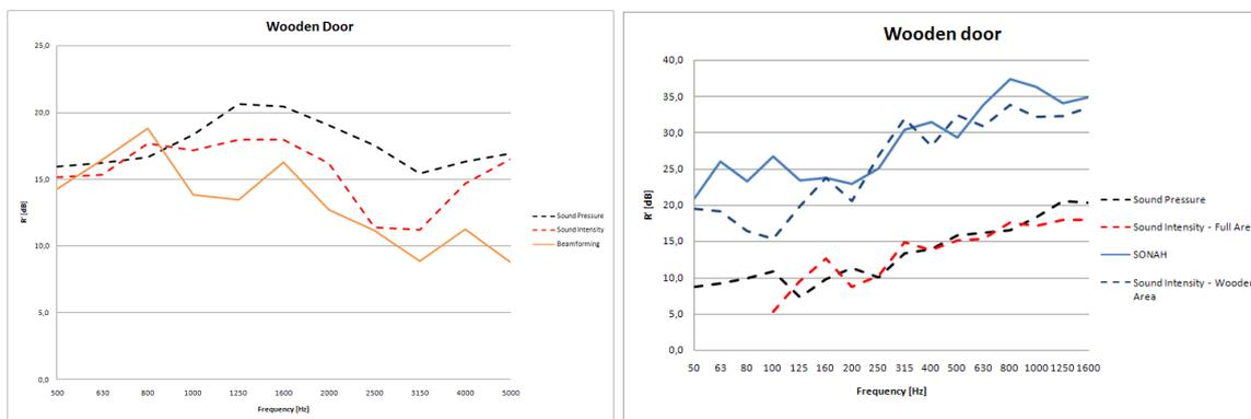
Figure 9: Comparison of sound reduction indexes for the wooden door. Left: Beamforming. Right: SONAH.
