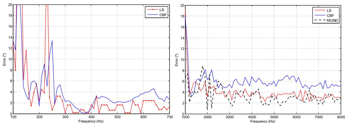
Figure 5: Error between estimated and real source location for the outdoor test (left) and the anechoic chamber experiment (right)
