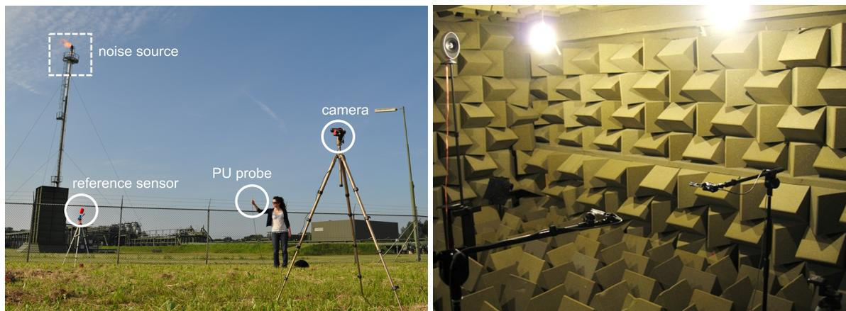
Figure 2: Pictures of the assessed measurement scenarios: outdoors experiment (left) and small anechoic chamber test (right)
