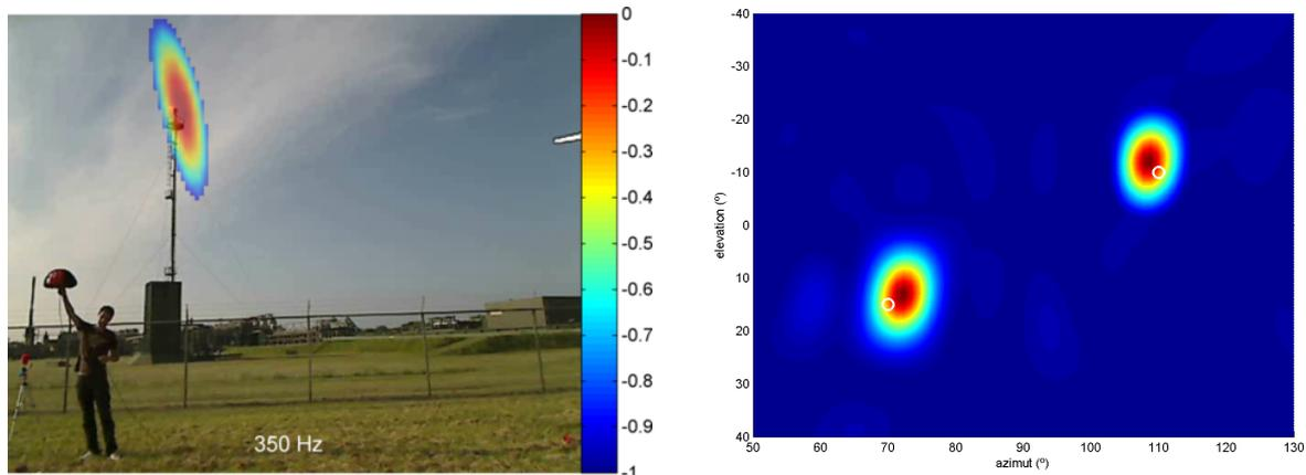
Figure 4: Least Squares localization map of the outdoor test at 350 Hz (left) and the anechoic chamber experiment at 5000 Hz (right)
