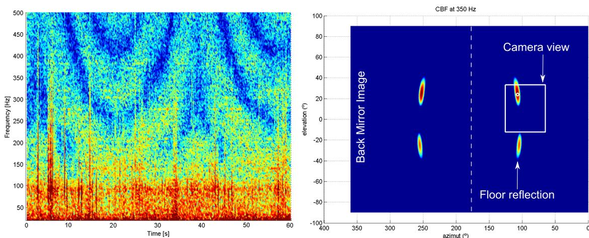
Figure 3: Spectrogram sample of the scanning sensor (left) and 360° localization map of the outdoor measurement (right)
