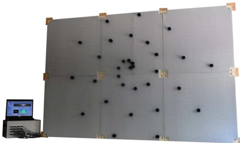
**Figure 7.1**      *Final acoustic camera prototype system.*
