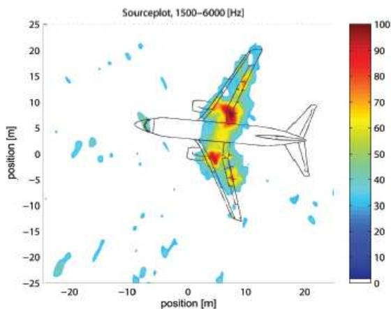
**Figure 6.5** Source plot of a Boeing 737.
