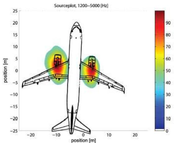
**Figure 6.6** Source plot of an Airbus A321.
