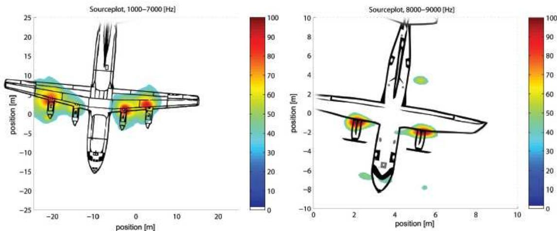
**Figure 6.1** Source plot of an Antonov AN-12. **Figure 6.2** Source plot of a Dornier 328.
