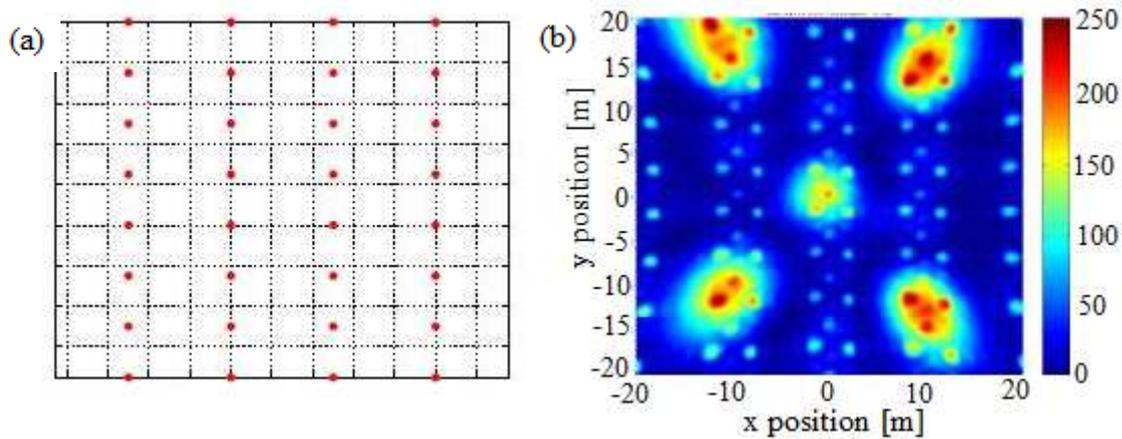
**Figure 5.3** (a) Microphone configuration and (b) source plot for a rectangular array.
