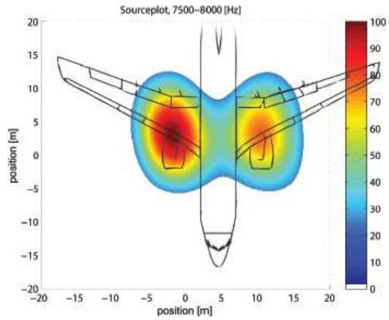
**Figure 6.4** Source plot of a Boeing 737.
