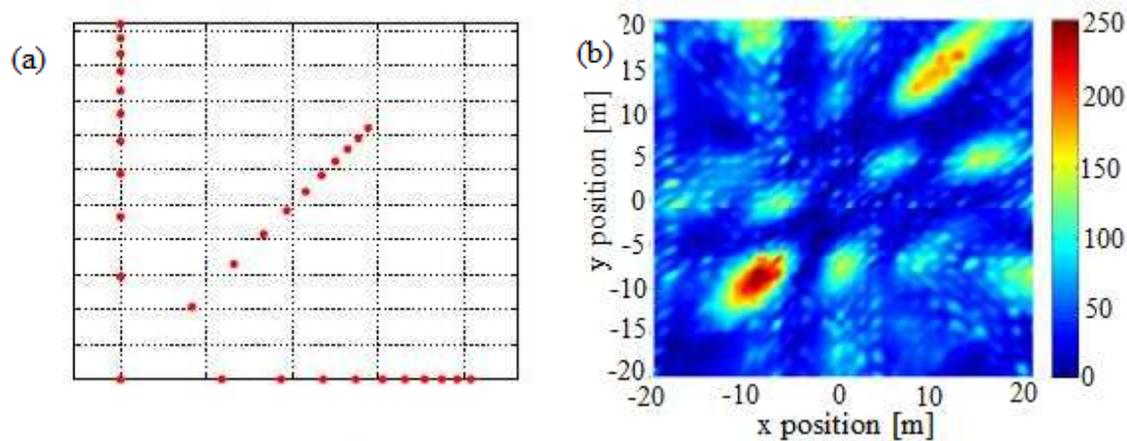
Figure 5.2 (a) Microphone configuration and (b) source plot for a logarithmic array.
