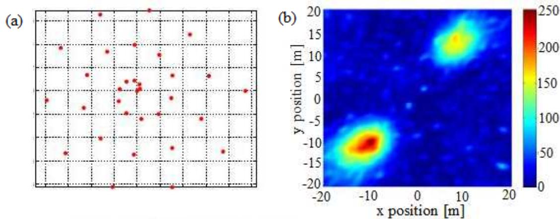
**Figure 5.4** (a) Microphone configuration and (b) source plot for a spiral array.
