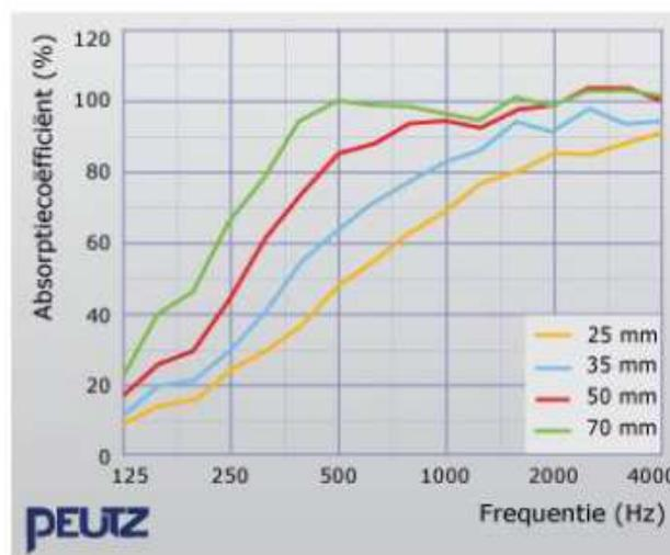
**Figure 2.2** Absorption coefficient versus frequency of the Flamex Basic foam used to reduce sound reflections of the wooden plates.
