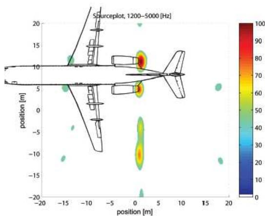
**Figure 6.7** Source plot of a Fokker 100.
