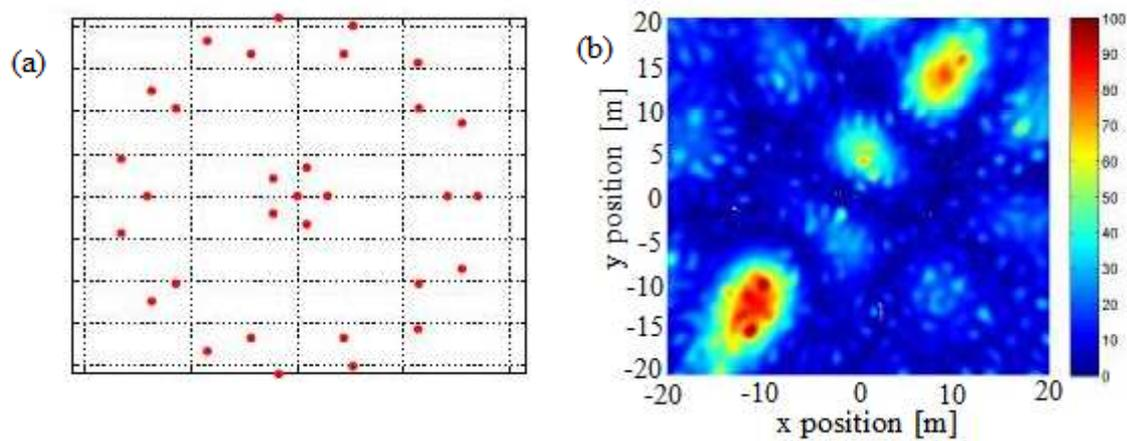
Figure 5.1 (a) Microphone configuration and (b) source plot for a circular array.
