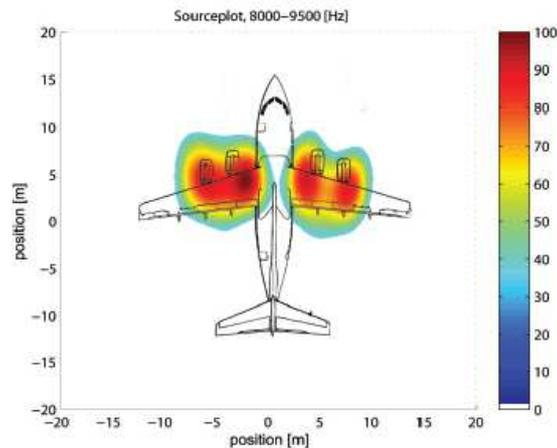
**Figure 6.8** Source plot of British Aerospace 146.
