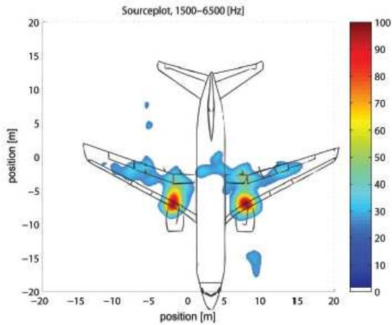
**Figure 6.3** Source plot of a Boeing 737.
