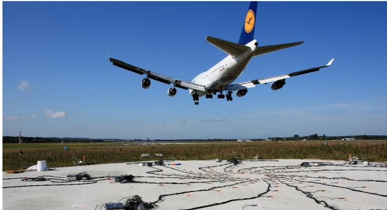
Figure 1: A Boeing 747 passing over a large microphone array set up by DLR for the fly-over measurements performed by DLR and Lufthansa in September 2008 at Parchim Airport
