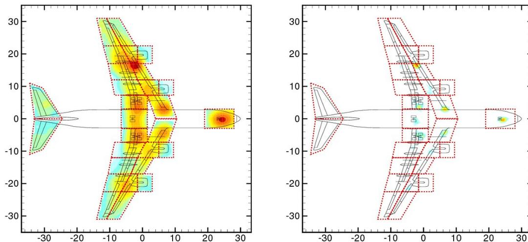
Figure 10: Source maps of an A340 in the 4 kHz one-third-octave band with a dynamic range of 15 dB; left: classical beamforming, right: deconvolution method.
