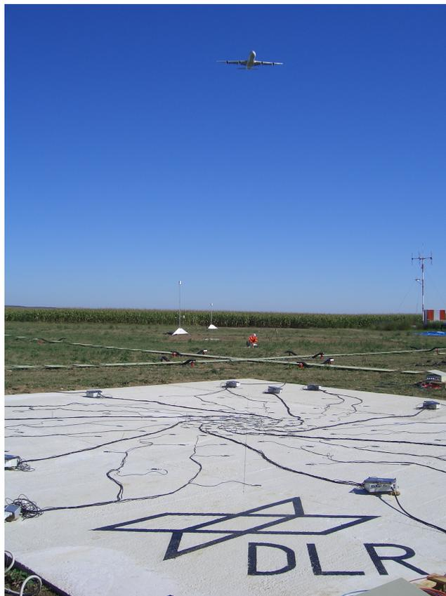
*Figure 3: The spiral microphone array of DLR and the cross array of ONERA used in the EU project AWIATOR in 2006.*
