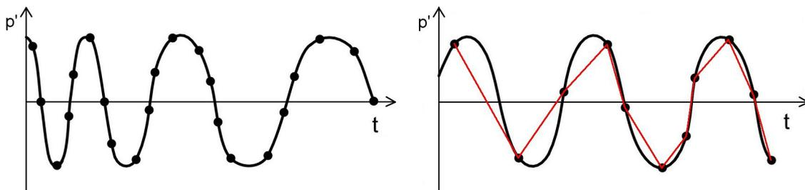
Figure 6: Compensation of the Doppler frequency shift at the microphone position by restoring the signal at the source at emission time  $t_e$ ; left: Doppler-shifted time series received at the microphone, sampled at constant time intervals; right: same time series re-ordered according to the emission time, re-sampling at constant time intervals will be on the basis of the original samples (black dots connected by the red line), not the original signal (black curve).
