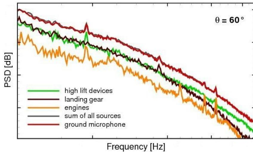
Figure 11: frequency spectra from the deconvolution analysis of the flyover in figure 10 for the reference microphone on the ground and for the integrated source regions at the high-lift devices, the landing gear and the engines.
