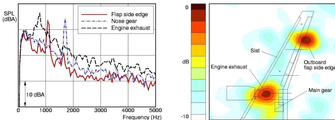
Figure 8: Sound sources on the wing of the A319; left: spectra from the beamforming analysis focused on the flap-side-edge, the nose gear, and the engine exhaust; right: a source map of the A319 wing in the 1 kHz one-third-octave-band (DLR data, analysed in cooperation with RWTH Aachen).
