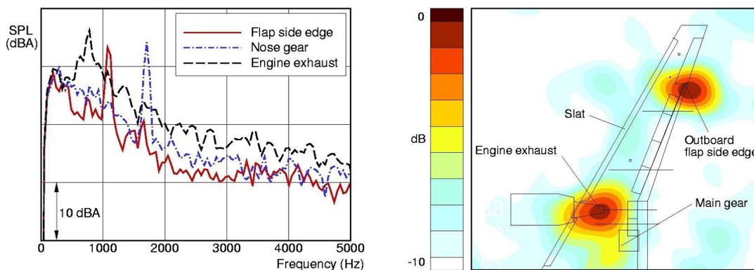
Figure 8: Sound sources on the wing of the A319; left: spectra from the beamforming analysis focused on the flap-side-edge, the nose gear, and the engine exhaust; right: a source map of the A319 wing in the 1 kHz one-third-octave-band (DLR data, analysed in cooperation with RWTH Aachen).
