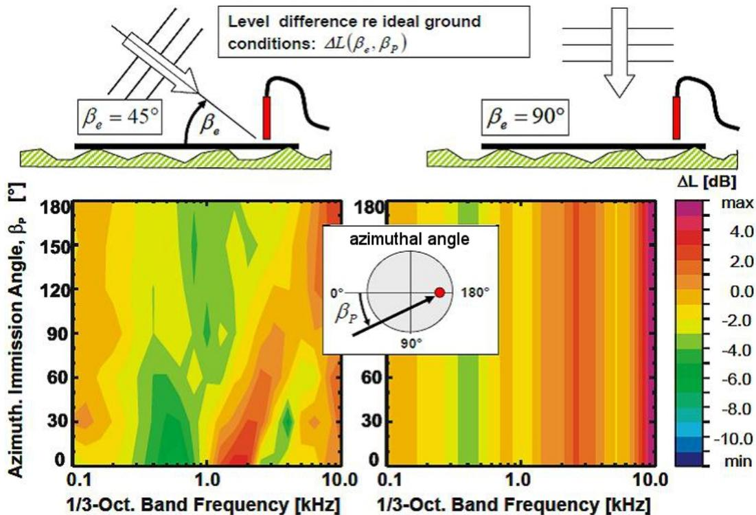
Figure 5: Directivity of a microphone on a ground plate [22]. Left: sound waves coming in from the side at an angle of  $\beta_e = 45^\circ$ ; right: sound from directly above the plate.
