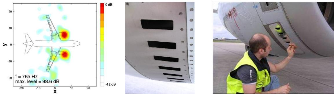
Figure 9: Modification of the de-icing system vent openings in the nacelle of the CFM56-5A engine that suppresses an 800 Hz tone; left: source map, centre: original vents, right: geometric modification.
