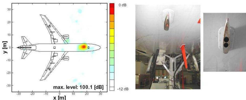
Figure 12: Cavity noise generated at the drain mast of the MD-11: left: sound source map in the 790 Hz one-third-octave band at  $\theta = 90^\circ$ ; center: view under the fuselage downstream of the nose landing gear; right: the drain mast with its two cavities
