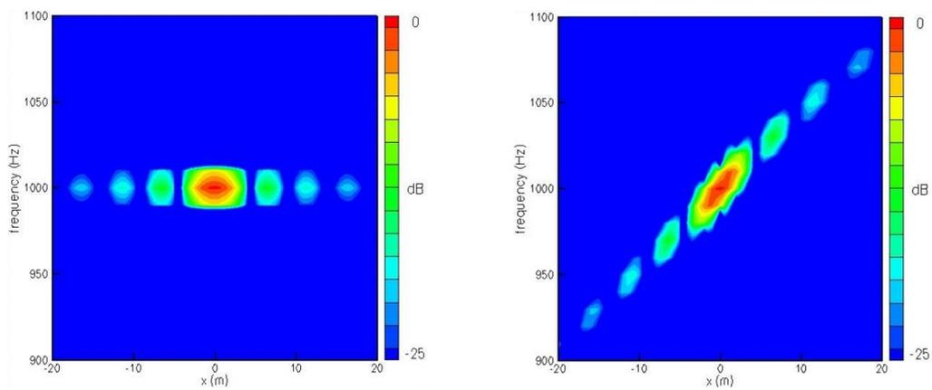
Figure 7: Point spread function of a linear microphone array as a function of the distance  $x$  parallel to the array and the frequency  $f$ ; for a stationary source (left) and for a moving source (right).
