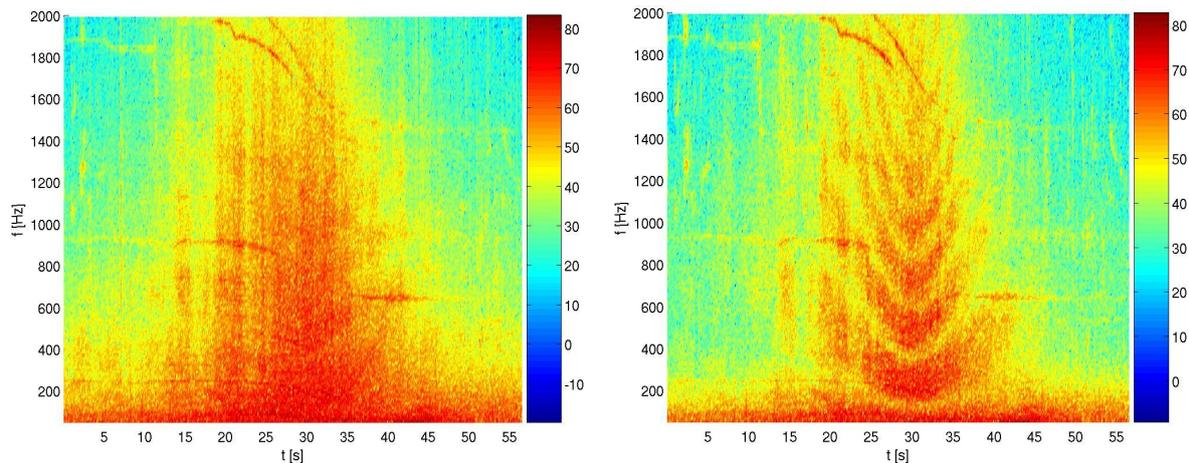
Figure 4: Spectrograms calculated from simultaneous recordings of one flyover with a ground microphone (left) and a microphone mounted 1.2m above ground (right).
