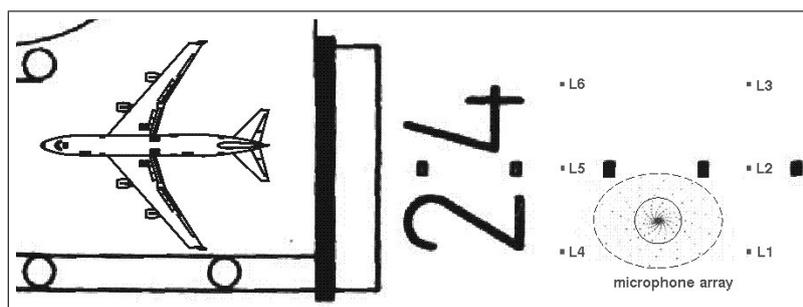
Figure 2: The set-up of the 43x36 m multi-arm spiral array for the B747 fly-over measurements of DLR and Lufthansa at Parchim airport, 2008; the aircraft on the runway is shown in order to indicate the relative size, the points L1–L6 mark the locations of the laser distance meters.
