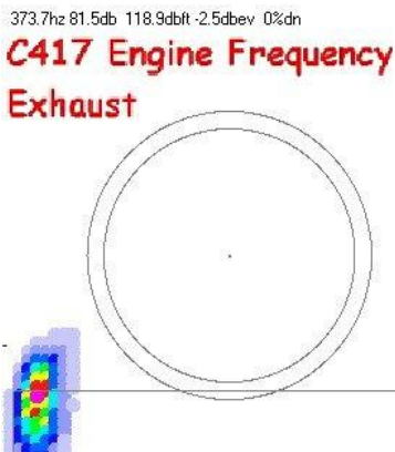
Fig8 Front view shows exhaust problem
