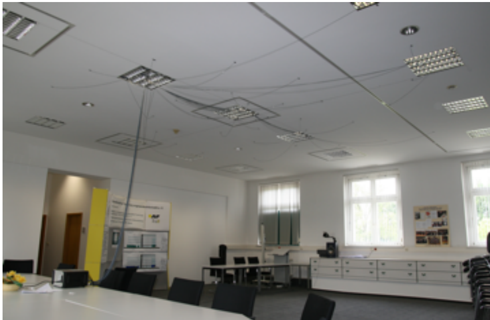
Fig. 5 spiral array (48 microphones, diameter approx. 6 m)
