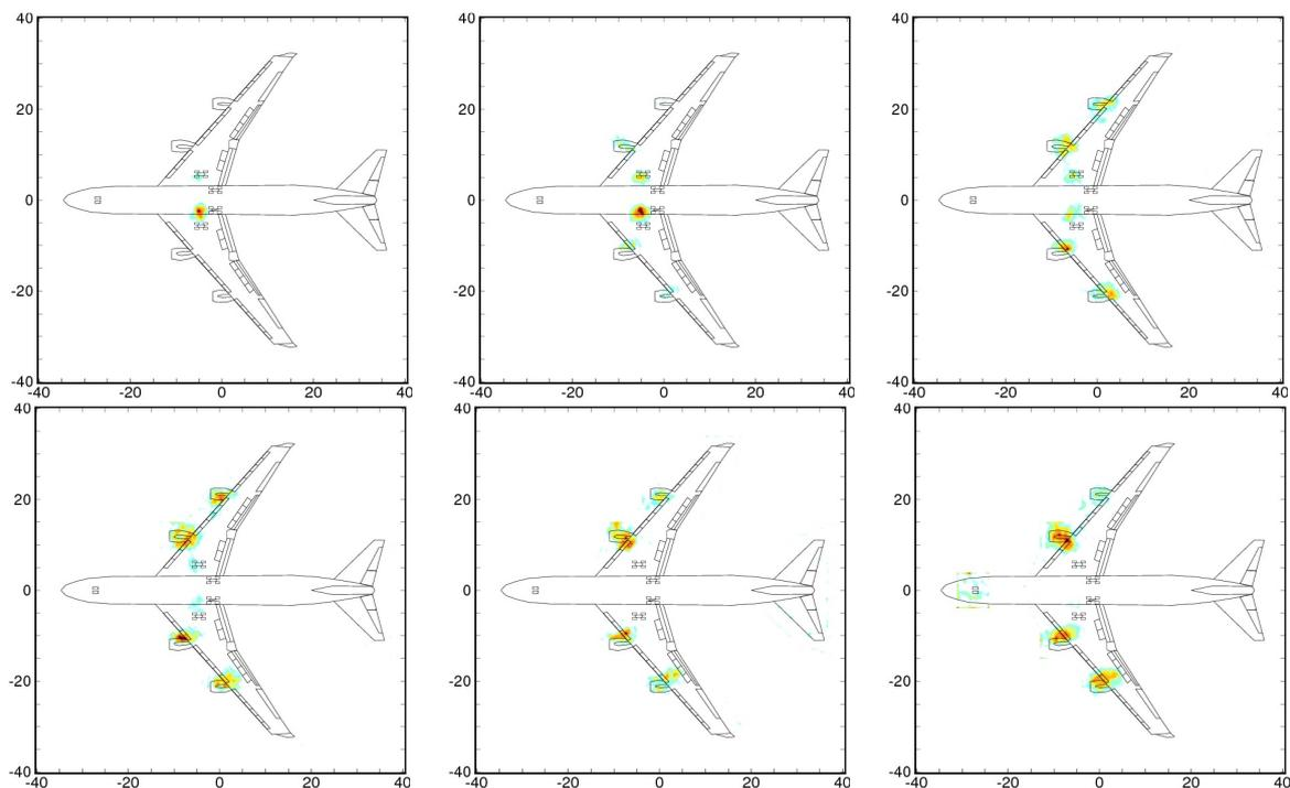
Figure 9: Results of the deconvolution analysis for a fly-over with extended landing gears from the high-frequency array;  $\theta = 90^\circ$ , 12 dB dynamic range, from left to right, top: 2500 Hz, 3150 Hz, and 4000 Hz; bottom: 5000 Hz, 6300 Hz, and 8000 Hz
