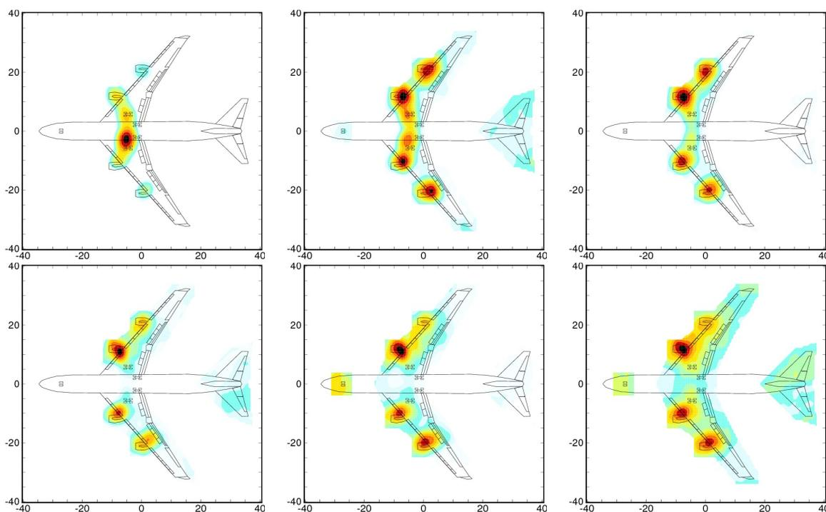
Figure 7: Results of the classical beamforming analysis for a fly-over with extended landing gears from the high-frequency array; from left to right, top: 3150 Hz, 4000 Hz, and 5000 Hz; bottom: 6300 Hz, 8000 Hz, and 10000 Hz
