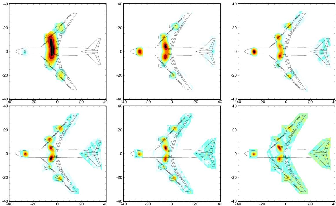
Figure 4: Results of the classical beamforming analysis for a fly-over with extended landing gears from the low-frequency array;  $\theta = 90^\circ$ , 10 dB dynamic range, from left to right, top: 200 Hz, 315 Hz, 400 Hz; bottom: 500 Hz, 630 Hz, and 800 Hz.
