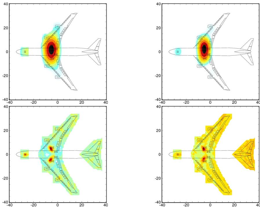
Figure 5: Results of the classical beamforming analysis for a fly-over with extended landing gears: overlap between the low- and the high-frequency arrays;  $\theta = 90^\circ$ , 10 dB dynamic range, left: 1000 Hz, right: 1250 Hz; top: high-frequency array, bottom: low-frequency array
