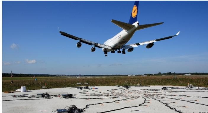
Figure 1: A Boeing 747-400 passing over a microphone array at Parchim airport (DLR, 2008)
