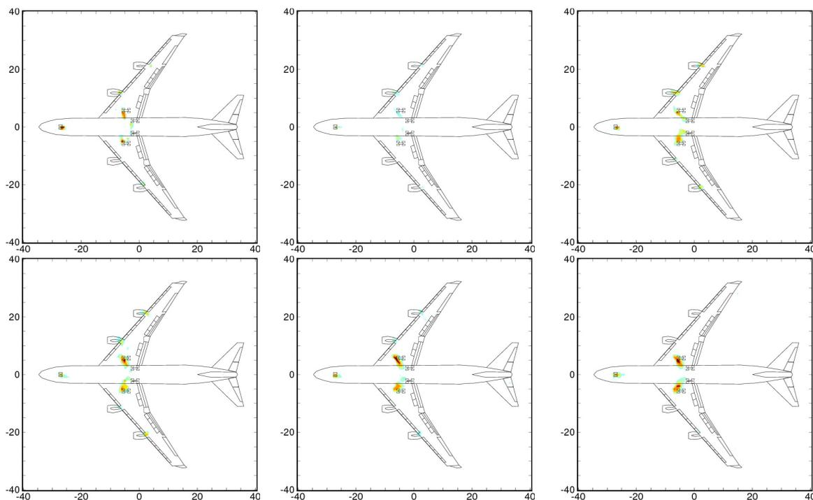
Figure 8: Results of the deconvolution analysis for a fly-over with extended landing gears from the lower frequency range;  $\theta = 90^\circ$ , 12 dB dynamic range, from left to right, top: 315 Hz, 400 Hz, and 500 Hz; bottom: 630 Hz, 800 Hz, and 1000 Hz
