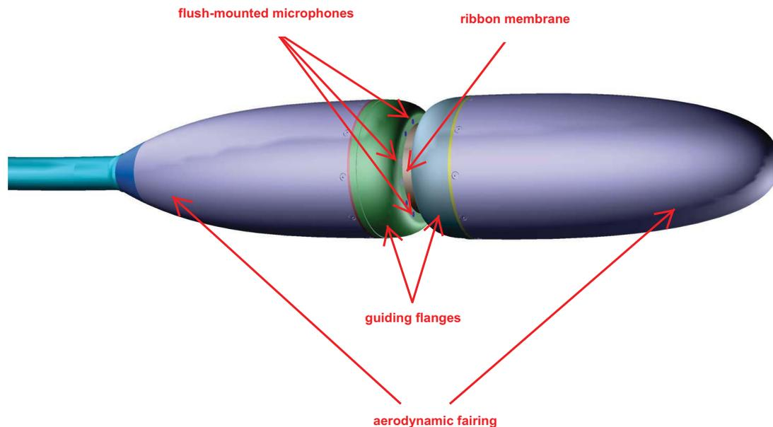
Figure 3: Sketch of the in-flow calibration sound source
