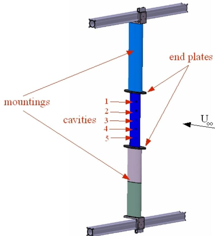
Figure 4: Sketch of the plate with cavities
