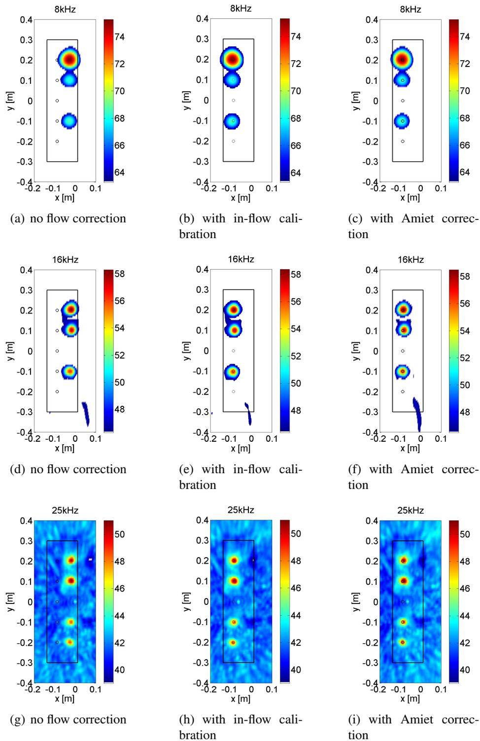
Figure 6: Beamforming results (in dB) of the plate with cavities for selected 1/3 octave bands for  $U_\infty = 50$  m/s without flow correction, with in-flow calibration and Amiet correction. The black box marks the position of the plate and the black circles the location of the cavities.
