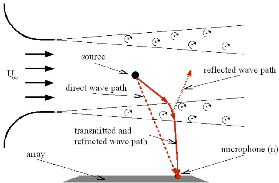
Figure 1: Schematic sketch for microphone array measurements in open jet wind tunnels
