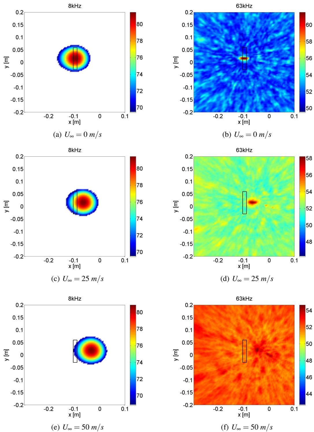
Figure 5: Beamforming results (in dB) without flow corrections of the in-flow calibration sound source for selected 1/3 octave bands for various flow velocities. The black box marks the position of the loudspeaker membrane.
