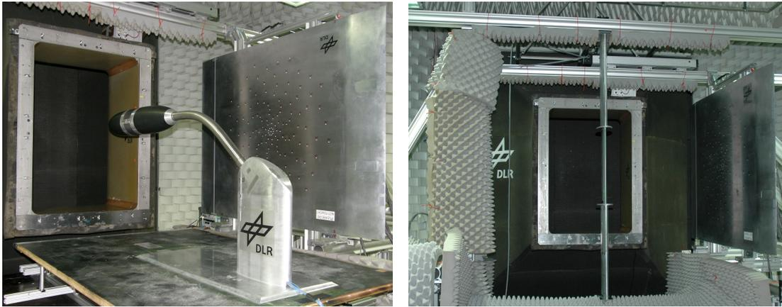
Figure 2: Installation of both models in the wind tunnel with the microphone array on the right side
