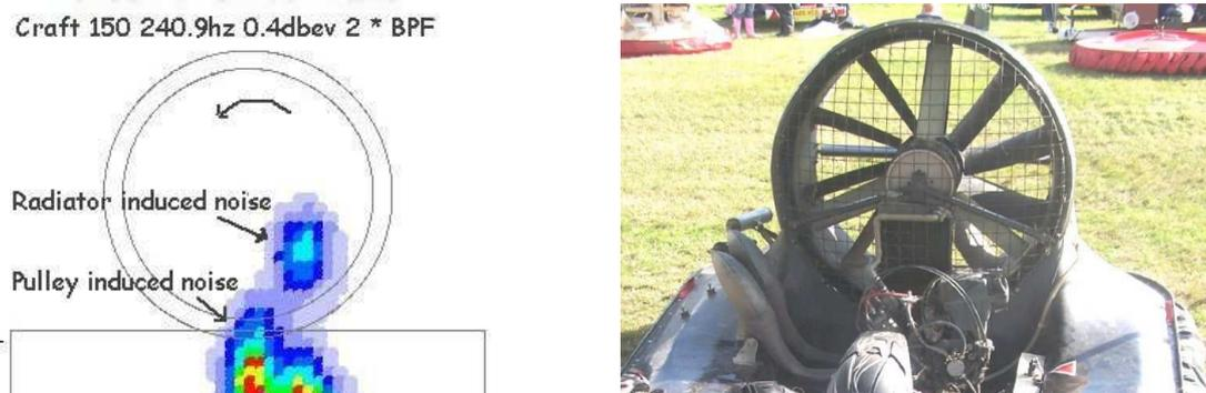
Fig.5. On this craft with a separate lift fan the 4<sup>th</sup> harmonic of the lift engine firing frequency is loudest. The engine air intake is louder than the exhaust outlet.
