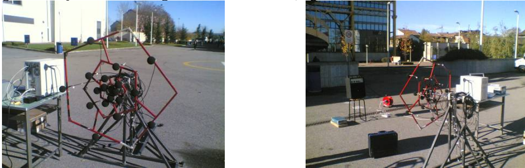
Fig. 10: View of the rotating pentagonal array (type C) and the measurement set-up
