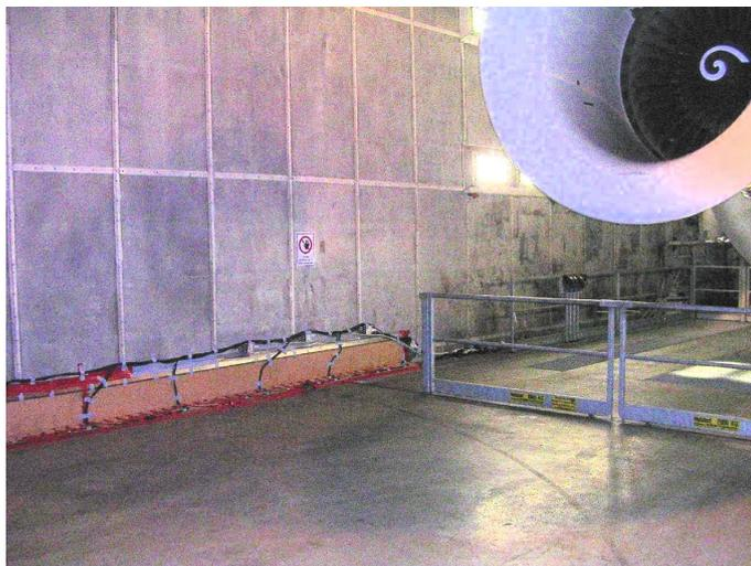
Figure 3: Linear microphone array along the side-wall of the test-cell
