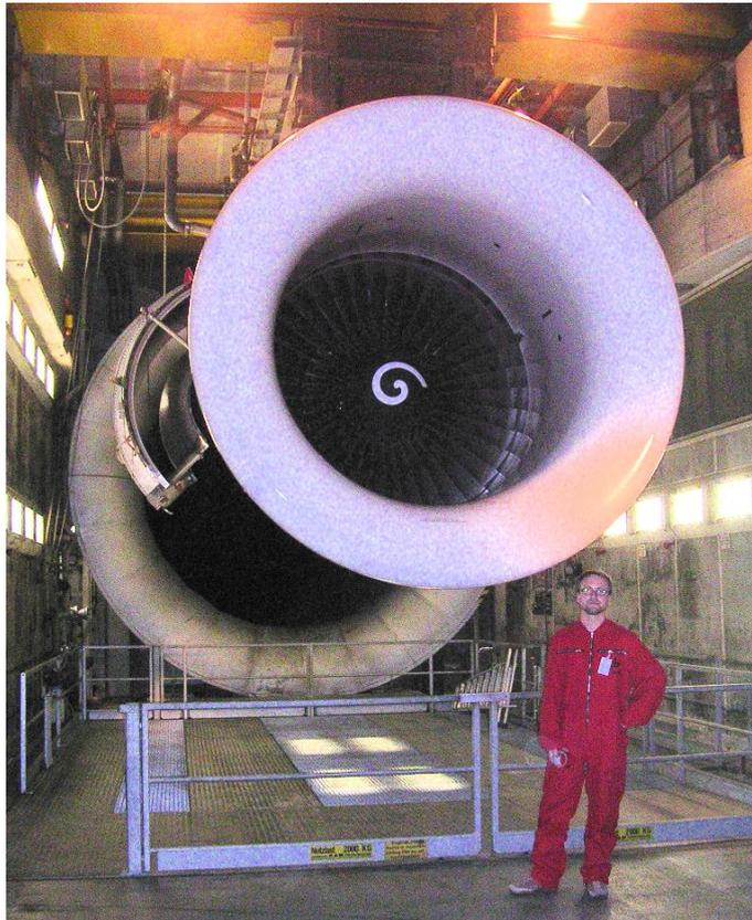
Figure 2: The engine with the bell-mouth inlet in the test-cell
