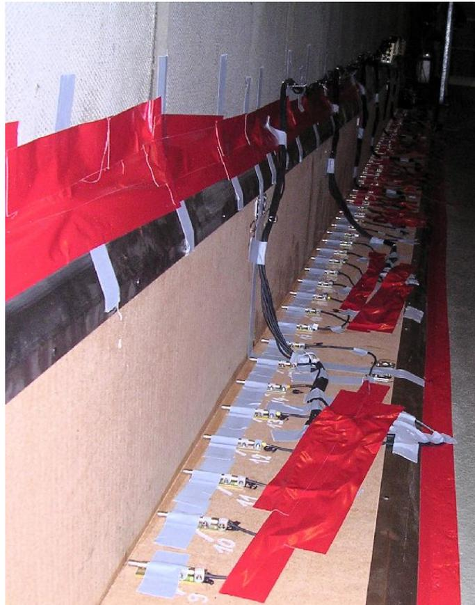
*Figure 4: Linear microphone array along the side-wall of the test-cell*
