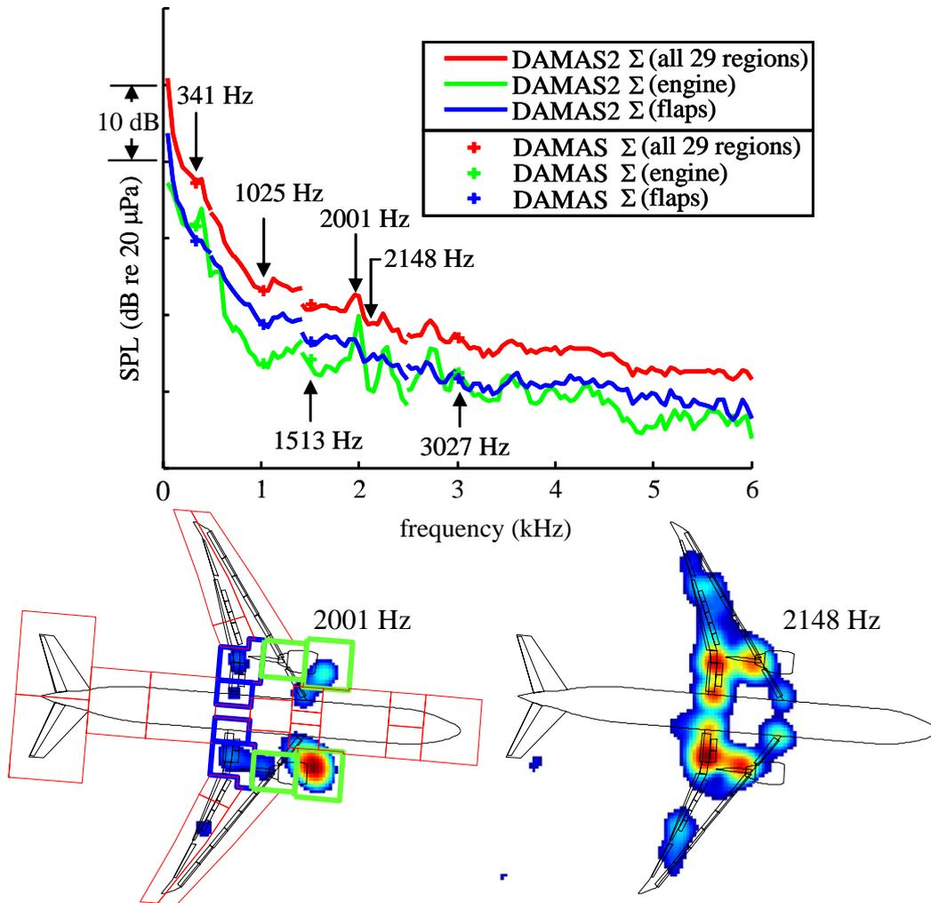
Fig. 4. Noise subcomponent spectra and sample conventional beamforming maps (beamform map colorbar same as in Fig. 1).
