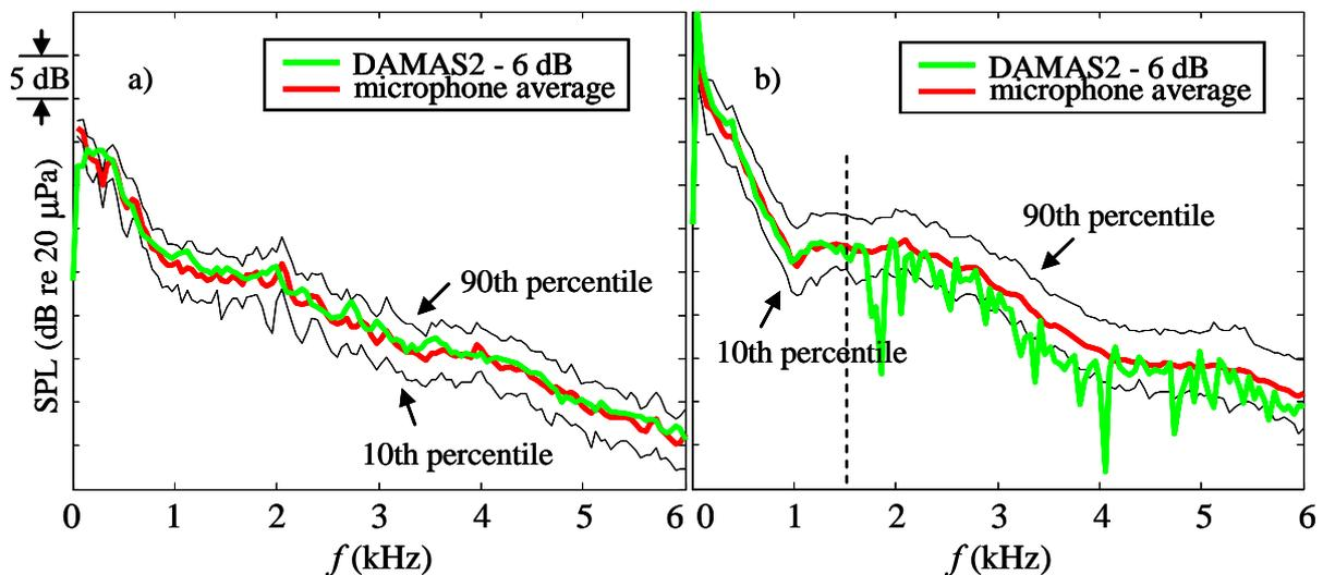
Fig. 5. a) High frequency array DAMAS2 comparison with microphone spectra – 7.6 m array *a*;
