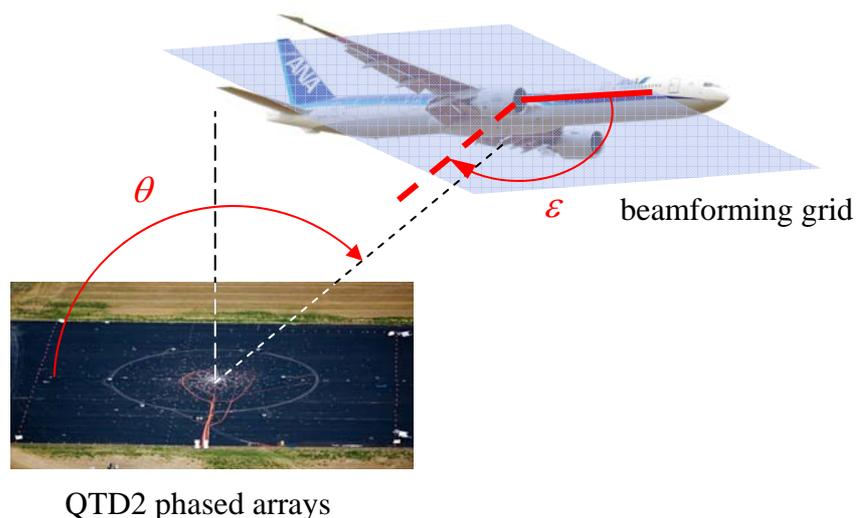
Fig. 3. QTD2 flight test geometry (aircraft bearing angle,  $\theta$ , and emission angle,  $\varepsilon$ ).
