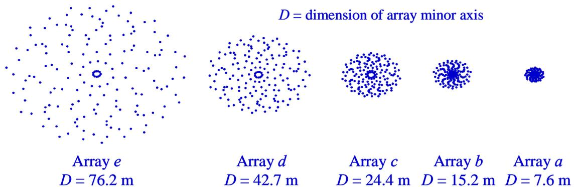
Fig. 2. QTD2 phased array microphone distributions (high frequency arrays *a*, *b*; low frequency arrays *c*, *d*, *e*).
