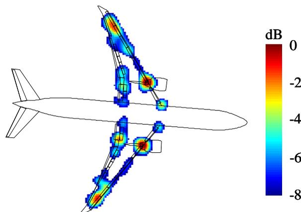
Fig. 1. Typical flight test aircraft noise sources, including airframe and engine related sources.
