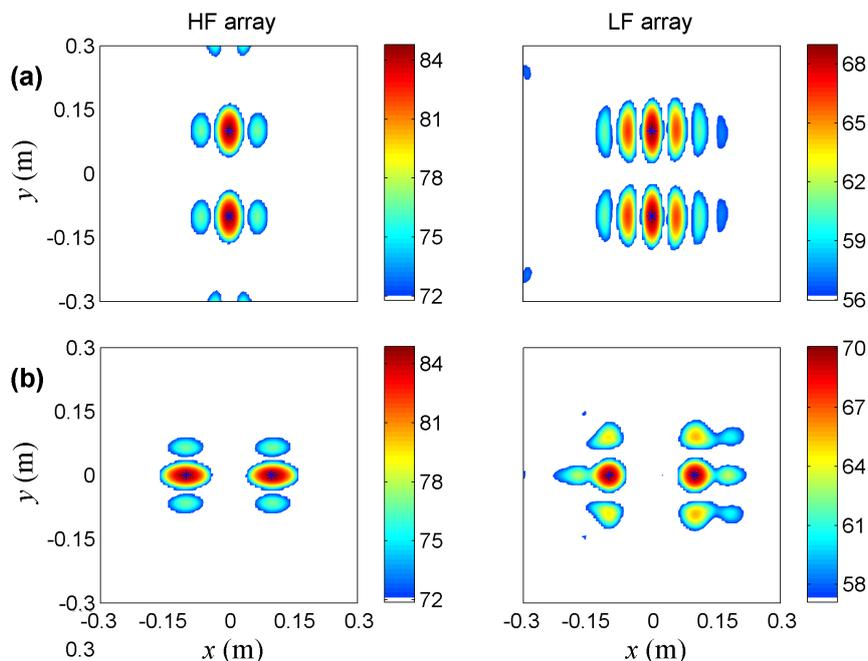
Figure 4: (Color online) Simulated multiple dipole sources by the D-Beam algorithm: (a) 2 X  $(1, 0, 0)$  dipoles located at  $(0.0, -0.1)$  and  $(0.0, 0.1)$ ; (b) 2 Y  $(0, 1, 0)$  dipoles located at  $(-0.1, 0.0)$  and  $(0.1, 0.0)$ . HF array,  $f = 12500$  Hz; LF array,  $f = 4000$  Hz.
