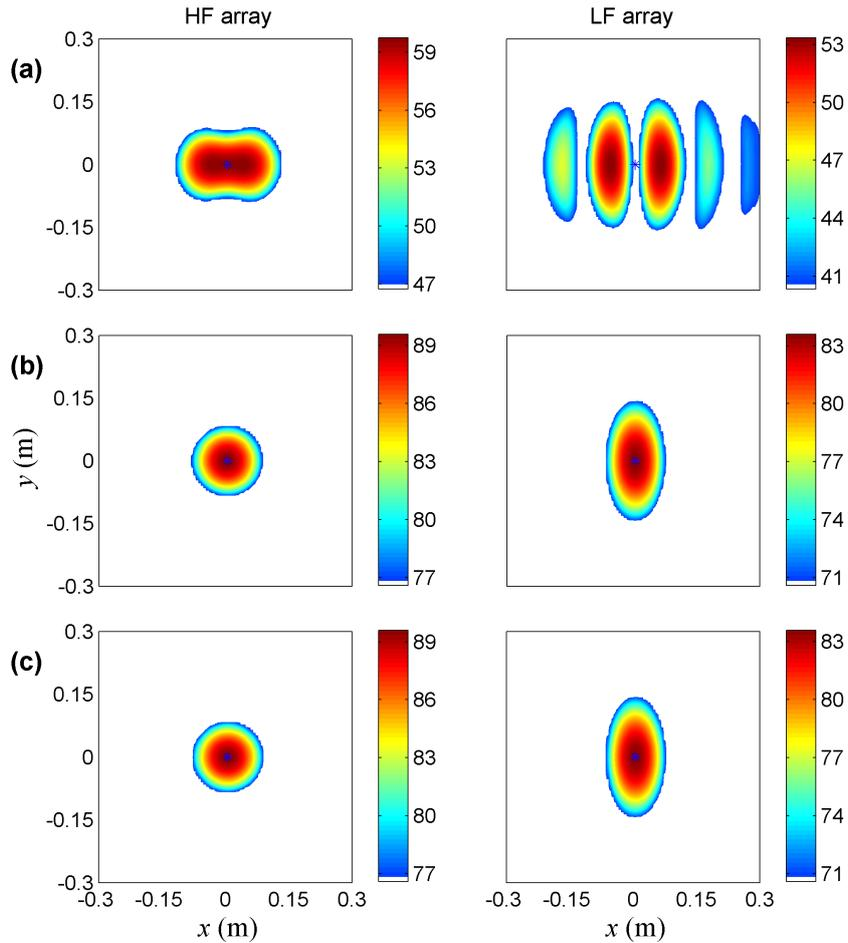
Figure 1: Simulated source maps for the X dipole: (a) dipole without correction; (b) dipole with signal correction; (c) reference monopole. HF array,  $f = 8000 \text{ Hz}$ ; LF array,  $f = 2000 \text{ Hz}$ .
