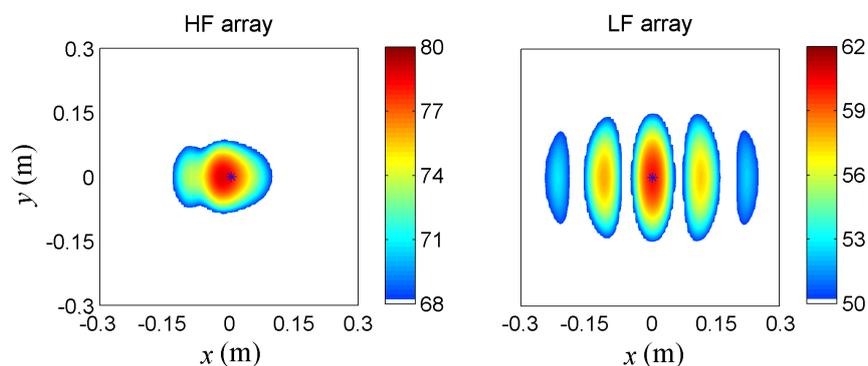
Figure 3: Simulated source maps by the D-Beam algorithm for the X dipole: HF array,  $f = 8000$  Hz; LF array,  $f = 2000$  Hz.
