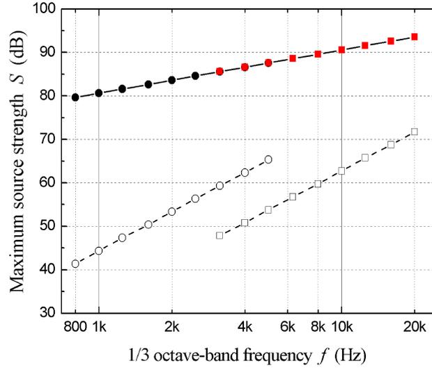
Figure 2: Variation of peak source power  $S$  with 1/3 octave-band centre frequency  $f$ : Dipole without correction:  $\square$  HF array,  $\circ$  LF array; dipole with signal correction:  $\blacksquare$  HF array,  $\bullet$  LF array;  $---$   $S \sim f^3$ ,  $---$   $S \sim f$ .
