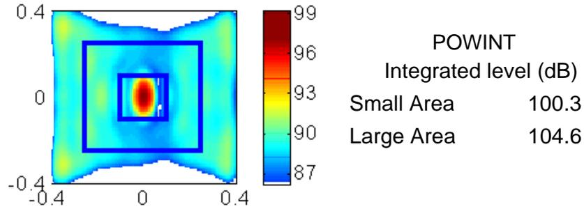
Figure 5 – Simulated background noise (101x101 grid of point monopole sources) with superimposed ‘model’ sources 10dB above (2x2 central grid).
