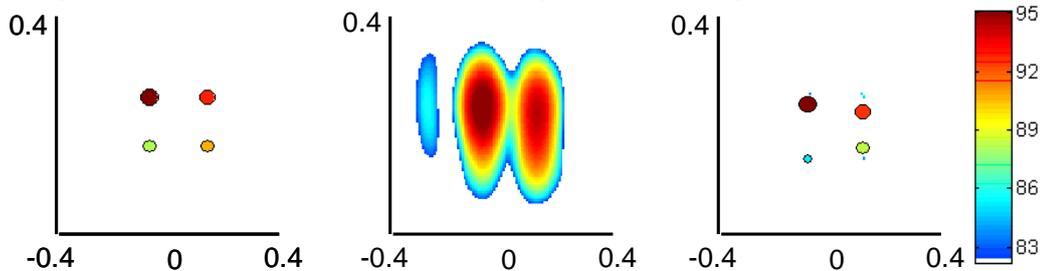
Figure 6 – (a) Simulation input (b) Beamforming (c) output from CLEAN
