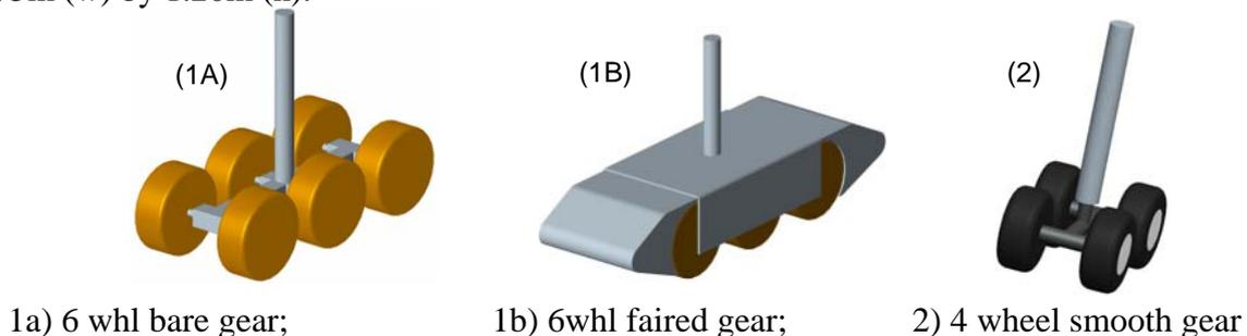
Figure 1: Models examined in the wind tunnel.
