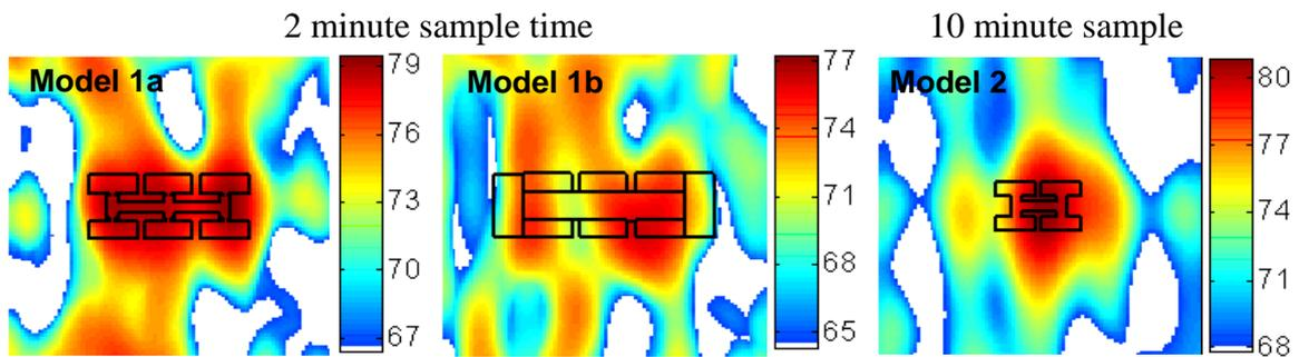
Figure 2 – Source autopower estimates for the models of figure 1, at 1250Hz.
