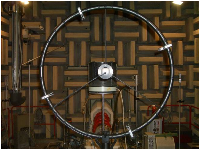
Fig.1. Positions 4 B&K 4190 Mic's on Ring
