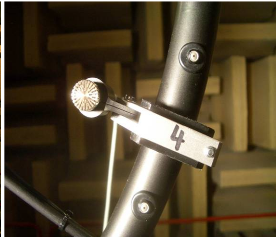
Fig.2. Detail Adapter of B&K Mic Nr.4
