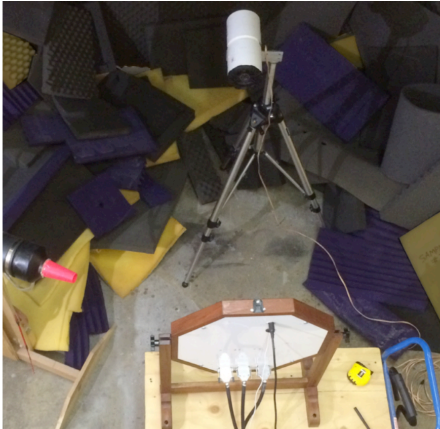
Fig. 1. Test setup. The phased array attempts to measure a broadband speaker source while a jet of air from the nozzle on the left impinges obliquely on the array face.
