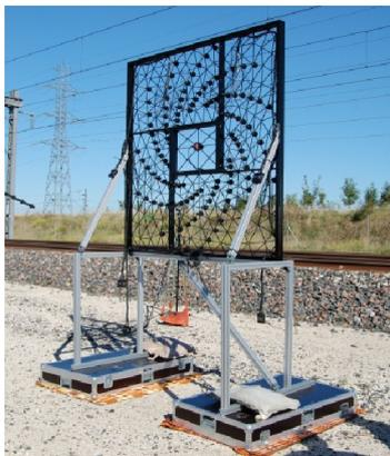
*Fig. 1 : Measurement setup with a 120 channel microphone array (spiral) with built-in industry camera*
