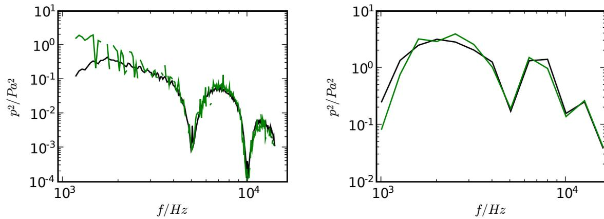
Figure 2: Example results for source spectra from lower left sector — from measurement with four loudspeakers — from measurement with single loudspeaker; auto power spectrum with  $\Delta f = 46.875$  Hz (left) third-octave spectrum (right)
