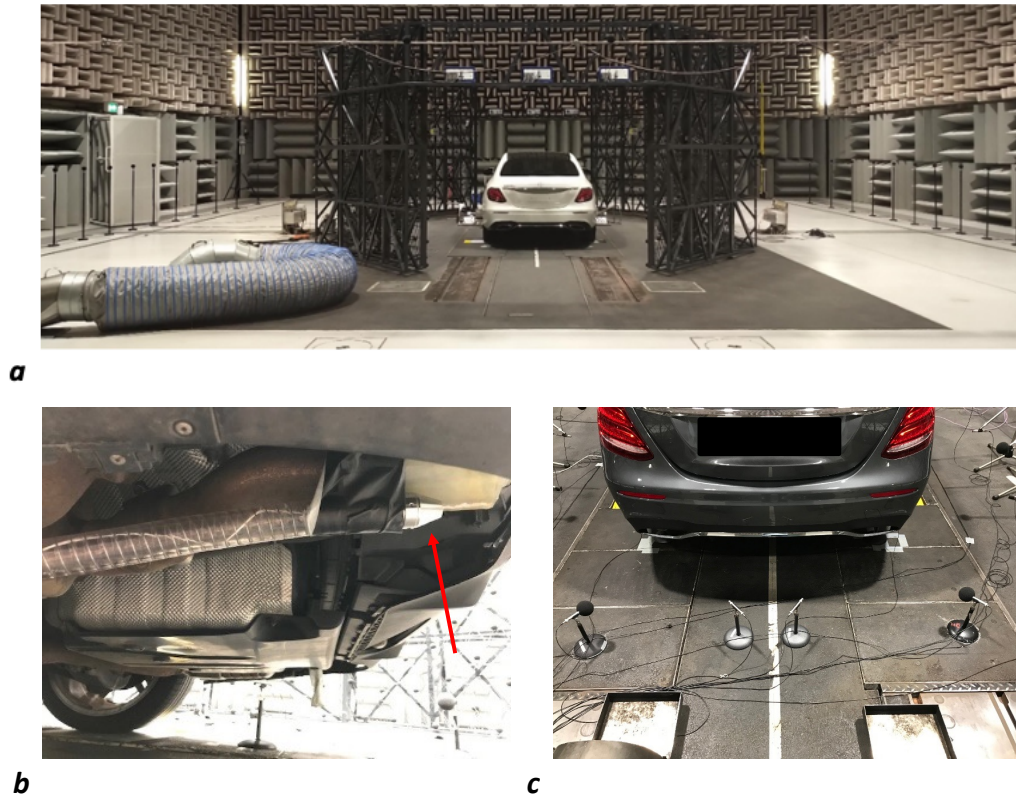
Fig. 4 Measurement arrangement on the indoor pass-by noise test track. a: Car placed on the dynamometer including the microphone array for HIBF (surrounding the car) and the microphone lines for simulated pass-by (at the left and right wall). b: VVS (red arrow) to measure the transfer functions. c: Indicator microphones for ASQ.
