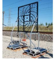
Fig. 1 : Measurement setup with a 120 channel microphone array (spiral) with built-in industry camera
