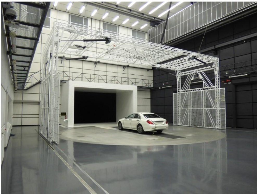
Fig. 1: The aeroacoustic wind tunnel of the Daimler AG. Two side and one top microphone array employing 360 microphones all together are used for the aeroacoustic car development [6].
