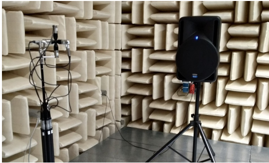
Figure 8: Measurement setup to measure the acoustic intensity with a PP-probe.
