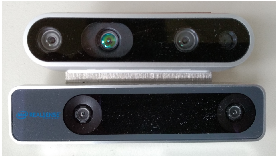
Figure 1: Intel Realsense D435 depth- (top) and T265 pose- (bottom) camera
