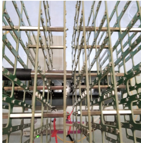
Figure 7: Measurement setup to measure the influence of the PP512 MEMS array on the acoustic field with a reference microphone.
