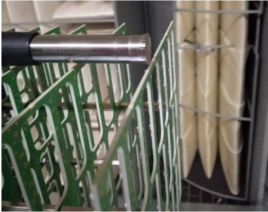
Figure 6: Measurement setup of the free field calibration procedure.
