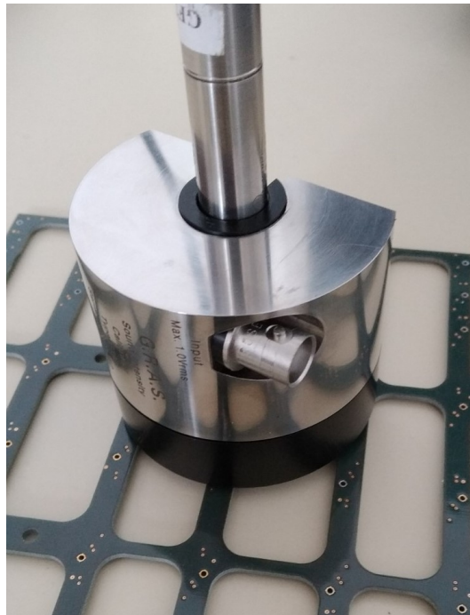
Figure 2: Measurement setup of the cavity calibration procedure
