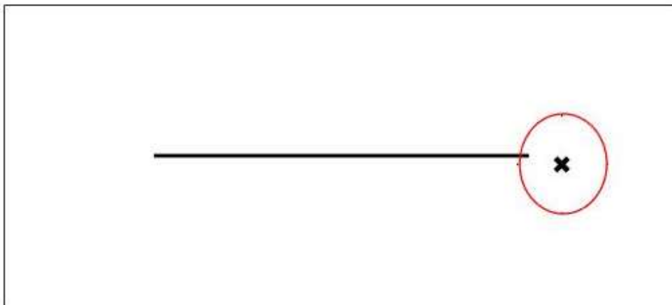
Figure 8. The average position of the detected trailing edge bluntness vortex shedding noise, with the indication of the standard deviation
