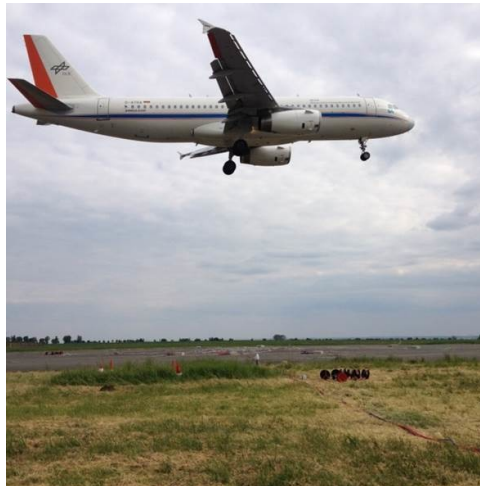
Figure 1: The DLR A320 research aircraft ATRA passing over the microphone array
