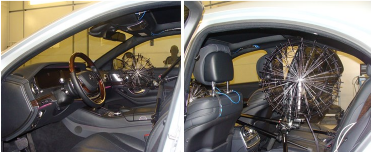
Figure 5: Positioning of the microphone arrays inside the vehicle interior
