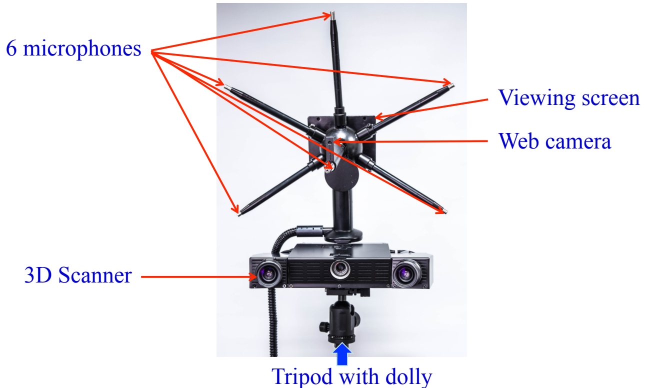
Figure 1. The major hardware involved in TSF V-Sonics include: 1) Six free-field probe microphones; 2) Two four-channel cDAQ by National Instruments; 3) One 3D scanner; 4) One viewing screen; 5) One web camera; 6) One laptop computer; 7) One tripod; and 8) One dolly.
