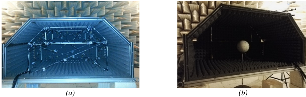
Fig. 2. A picture of the car cabin mock-up with trimming material attached to the walls: (a) distributed and (b) spherical array
