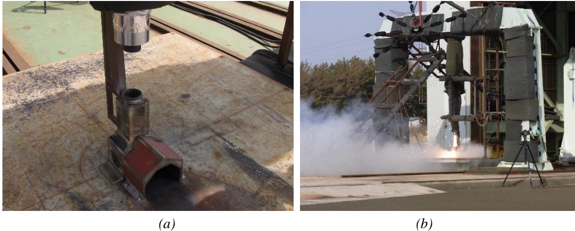
Fig. 6. (a): Subscale Rocket Motor and Launch Pad Model on Flat Plate. (b): Gate-Type Test Stand for SMAP-3 Including Microphone Array.
