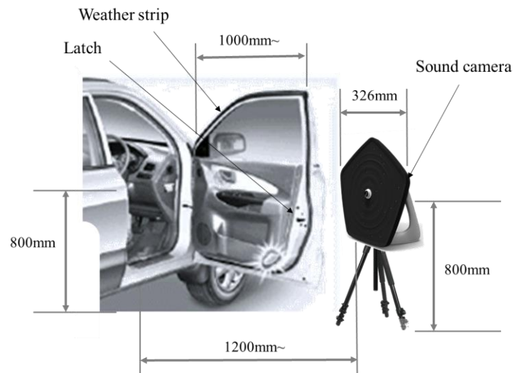
Fig. 4: The practical measurement configuration of door-slam sound with a microphone array. A commercial microphone array (SeeSV-S205) with 30 microphones and 326 mm diameter is located 1.2m away from the door.
