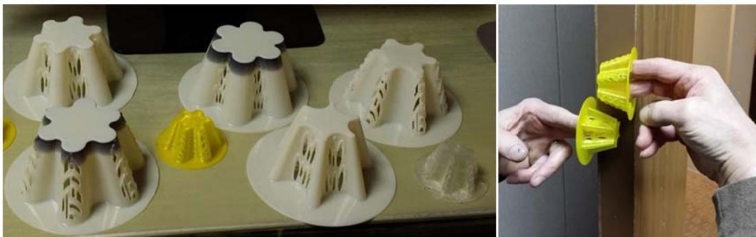
Figure 12 . Design detail and the proposed location of sound absorber or silencers within the door cavity.
