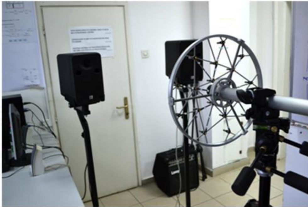
Fig.5 Measurement setup with Brüel & Kjær acoustic camera
