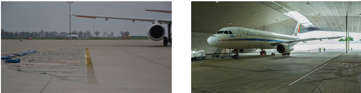
Figure 1: Set-up of the linear microphone array at the Cochstedt airfield (left) and in the engine test hangar of Lufthansa Technik at Hamburg airport (right).
