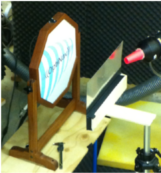
Figure 3: Test setup with an OptiNav 24 Jr microphone array[9].
