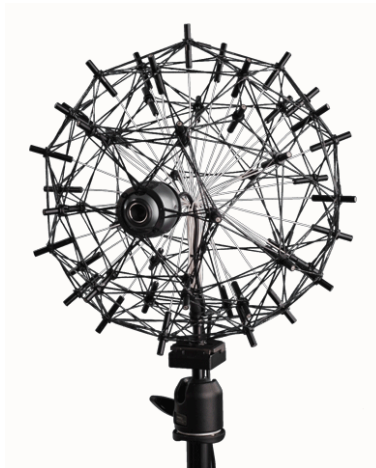
Figure 1: Spherical 48-channel transparent microphone array used for the RIR estimation.
