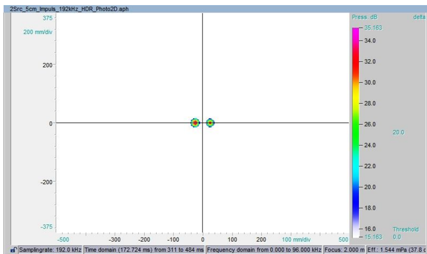
Fig. 11 Geometric resolution, 2 sources, 5cm distance, 2m focus distance, 20 dB mapping dynamic
