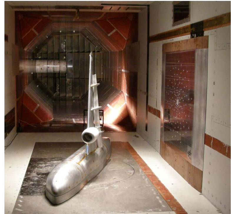
DO-728 half model in landing configuration
